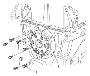
4. Remove the rear oil seal slinger (1).
