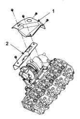
10. Remove the turbocharger assembly (1) from the cylinder head.
