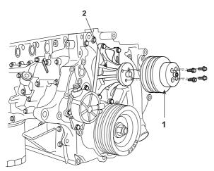
4. Remove the vacuum pump (1) and alternator assembly (2).
