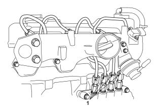
4. Loosen the hexa-bolt (2) of injector nozzle bridge (1) and remove the injector (3).
