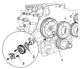
Install the supply pump gear.
