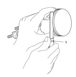
4. After installing the piston ring to the cylinder bore, push the piston ring to the vertical direction with the piston.
