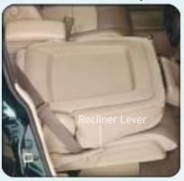
The front passenger seat can be folded flat. Pull up on the recliner lever, to the full upward position, to fold down the seat back.
