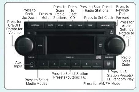
• The radio sales code is located on the lower right side of the radio faceplate.
