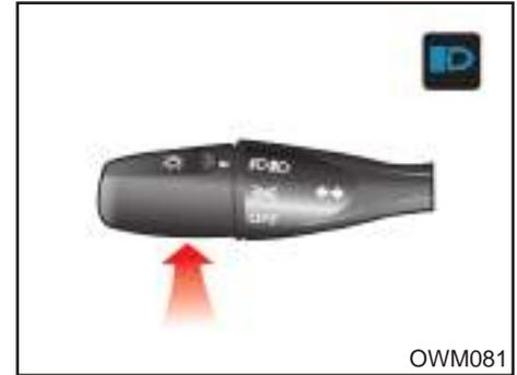
To set the headlamps in high-beam condition, push forward the control lever.
