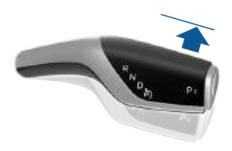
To re-enable cruising at the current driving speed, move the gear lever fully down once then release.
