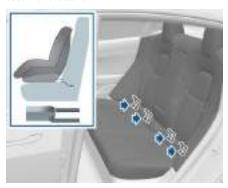
Once installed, test the security of the installation before seating a child. Attempt to twist the child safety seat from side to side and try to pull it away from the seat, then check to ensure the anchors remain securely in place.
