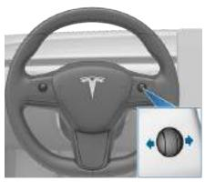
To display and adjust the setting for the following distance on the touchscreen at any time, touch Controls > Autopilot > Cruise Follow Distance. Adjust the following distance by touching plus (+) or minus (-) buttons.
