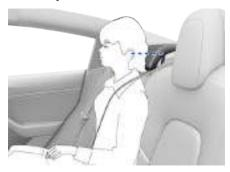
The head support in the rear center seat should always be lowered when a seat belt retained child safety seat is installed. See Raising/Lowering the Rear Center Head Support on page 19.
