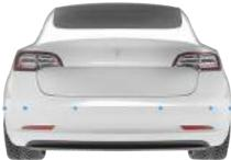
The sensors are activated when driving slower than 5 mph (8 km/h).
