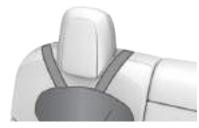
For single-strap tethers at the outboard seating positions, run the strap over the outside-facing side of the head support (i.e. same side of the head support as the seat belt retraction mechanism).
