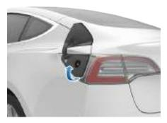
Note: The Tesla "T" lights up white when you open the charge port door. If you do not insert a charge cable into the charge port within a few minutes after opening the charge port door, the charge port door closes. If this happens, use the touchscreen to open the charge port door again
