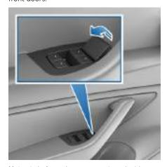
Note: Only front doors are equipped with a manual door release.
