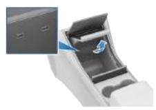
Two additional USB ports are located in the rear of the center console. Passengers in the rear seats can use these ports to charge their USB-connected devices. Media Player does not communicate with the rear USB ports.
