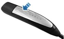
You can also open the charge port door using any of these methods:
