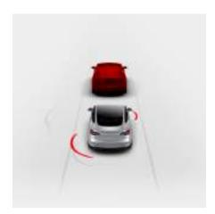
Warnings cancel automatically when the risk of a collision has been reduced (for example, you have decelerated or stopped Model 3, or the object in front of your vehicle has moved out of your driving path).
