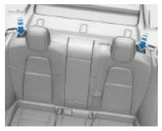
To fold a rear seat, pull the corresponding lever and fold the seat forward.
