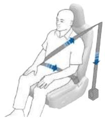
If the pre-tensioners and airbags did not activate in an impact, this does not mean they malfunctioned. It usually means that the strength or type of force needed to activate them was not present.
