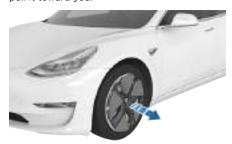
To install an aero cover, align it into position so that the notch is aligned with the tire's valve stem and then push firmly around its perimeter until it fully snaps into place.
