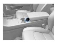
Note: You must position the key card within an inch or two of a card reader to allow Model 3 to read it. You may need to physically touch the center console or driver's side door pillar with the key card, and you may need to hold it against the transmitter for one or two seconds.
