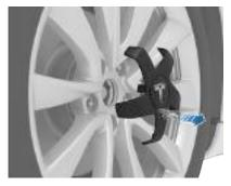
To install the lug nut cover, align it into position and push firmly until it fully snaps into place.
