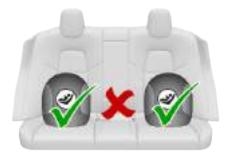
To install a LATCH child safety seat, slide the safety seat latches onto the anchor bars until they click into place. Carefully read and follow the instructions provided by the child safety seat manufacturer.
