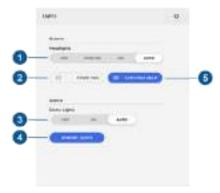
Exterior lights (headlights, tail lights, side marker lights, parking lights, and license plate lights) are set to AUTO each time you start Model 3. When set to AUTO, exterior lights automatically turn on when driving in low lighting conditions. If you change to a different setting, lights always revert to AUTO on your next drive.
