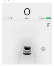
Note: The parking icon appears only if the vehicle's position and/or the circumstances of the surrounding area are such that Autopark can determine an appropriate driving path. If Autopark cannot determine an appropriate path (for example, when driving on a narrow street where moving into the parking space causes the front of the vehicle to extend into the adjacent lane), you can either reposition the vehicle, find a different parking space, or park manually.
