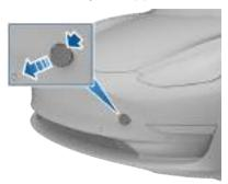
**3.** Pull the two wires out of the tow eye opening to expose both terminals.
