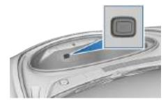
Press the interior release button to open the front trunk, then push up on the hood.
