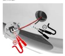
**Note:** Applying external 12V power to these terminals only releases the hood latches. You cannot charge the 12V battery using these terminals.
