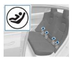
Install LATCH child safety seats in the outboard seating positions only. Use only a seat belt retained seat in the center position.
