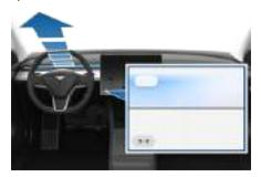
You can toggle between having the air flow from the vent in a single direction (represented on the control grid by an oblong shape) or in two mirrored directions (represented on the control grid by two circles). To do so, touch the combine/split icon. The icon changes based on whether air flow is combined or solit.
