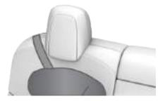
For a single-strap tether in the center seating position, fully lower the head support (see Raising/Lowering the Rear Center Head Support on page 19) and run the strap over the top center of the head support.
