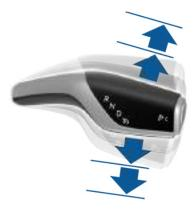
If you try to shift into a gear that the current driving speed prohibits, a chime sounds and the gear does not change.
