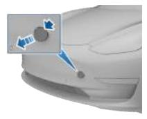
4. Fully insert the tow eye into the opening, then turn it counter-clockwise until securely fastened.
