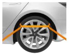
Caution: Attaching tie-down straps to the chassis, suspension or other parts of the vehicle's body may cause damage.
