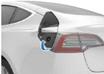
**Note:** The Tesla "T" lights up white when you open the charge port door. If you do not insert a charge cable into the charge port within a few minutes after opening the charge port door, the charge port door closes. If this happens, use the touchscreen to open the charge port door again
