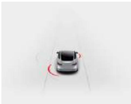
Lane Assist also warns you of undesired lane departures by vibrating the steering wheel slightly if a front wheel passes over a lane marking and the associated turn signal is off. This warning is active only when driving between approximately 36 and 90 mph (59 and 150 km/h). To turn this warning on or off, touch **Controls > Autopilot > Settings > Lane Departure Warning**. Your chosen setting is retained until you manually change it.
