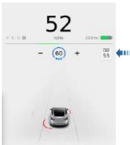
In situations where Speed Assist is unable to determine a speed limit (for example, speed limit signs and GPS data are not available at the current location), or if Speed Assist is uncertain that an acquired speed limit is accurate (for example, although a speed limit sign was initially detected, some time has passed before a subsequent sign has been detected), the touchscreen may not display a speed limit sign and warnings do not take effect.
