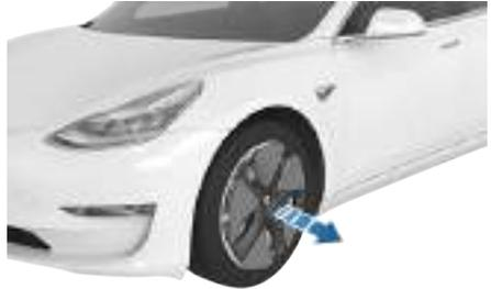
To install an aero cover, align it into position so that the notch is aligned with the tire's valve stem and then push firmly around its perimeter until it fully snaps into place.
