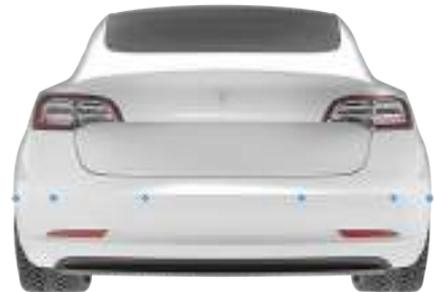
The sensors are activated when driving slower than 5 mph (8 km/h).
