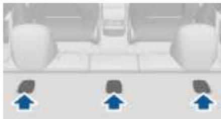
To access an anchor point, press down on the back of its cover.
