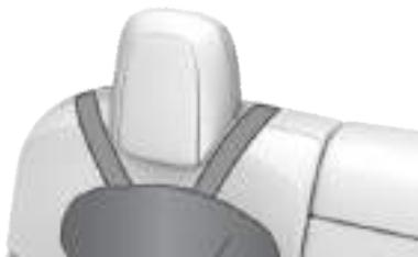
For single-strap tethers at the outboard seating positions, run the strap over the outside-facing side of the head support (i.e. same side of the head support as the seat belt retraction mechanism).
