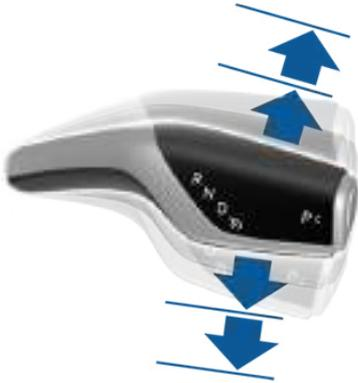
If you try to shift into a gear that the current driving speed prohibits, a chime sounds and the gear does not change.
