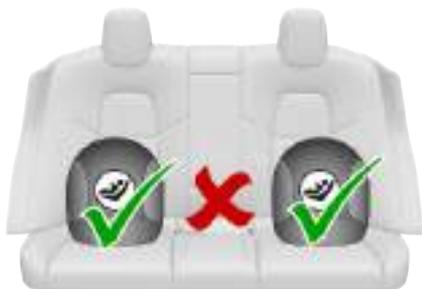
To install a LATCH child safety seat, slide the safety seat latches onto the anchor bars until they click into place. Carefully read and follow the instructions provided by the child safety seat manufacturer.
