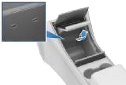
Two additional USB ports are located in the rear of the center console. Passengers in the rear seats can use these ports to charge their USB-connected devices. Media Player does not communicate with the rear USB ports.
