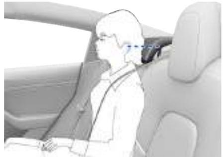
The head support in the rear center seat should always be lowered when a seat belt retained child safety seat is installed. See [Raising/Lowering the Rear Center Head Support](#) on page 19.
