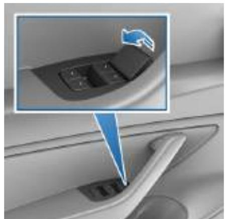
**Note:** Only front doors are equipped with a manual door release.
