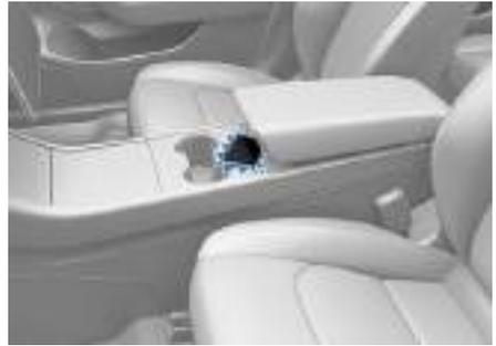
**Note:** You must position the key card within an inch or two of a card reader to allow Model 3 to read it. You may need to physically touch the center console or driver's side door pillar with the key card, and you may need to hold it against the transmitter for one or two seconds.
