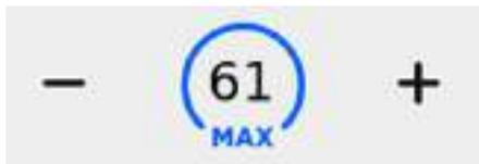
To cruise at the speed limit that is currently being determined by Speed Assist (including any offsets that you have set), move the gear lever fully down once then release. See [Speed Assist](#) on page 82.
