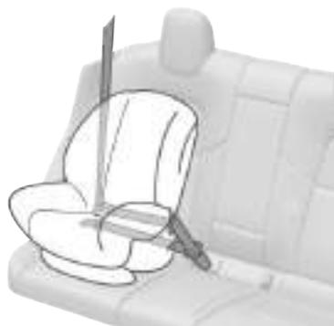
2. Allow the seat belt to retract, and remove all slack in the seat belt while firmly pushing the child safety seat into the Model 3 seat.
