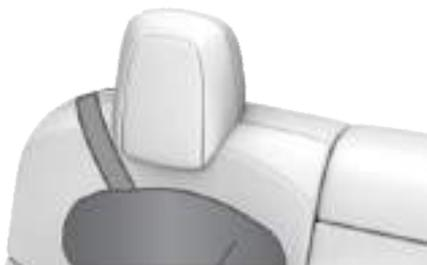
For a single-strap tether in the center seating position, fully lower the head support (see [Raising/Lowering the Rear Center Head Support](#) on page 19) and run the strap over the top center of the head support.
