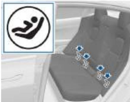
Install LATCH child safety seats in the outboard seating positions only. Use only a seat belt retained seat in the center position.
