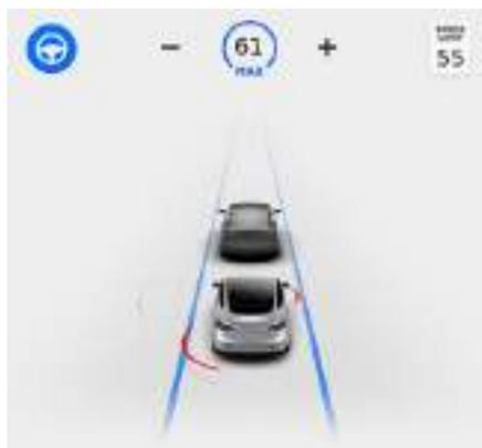
**Note:** To initiate Autosteer when there is no vehicle in front of you, you must be driving at least 18 mph (30 km/h) on a roadway with visible lane markings. If a vehicle is detected ahead of you, you can initiate Autosteer at any speed, even when stationary (if you are at least 5 feet (150 cm) away from the vehicle).
