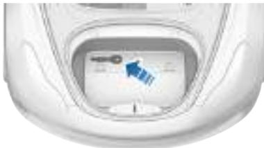
3. Release the tow eye cover by pressing firmly on the top right perimeter of the cover until it pivots inward, then gently pulling the raised section toward you.
