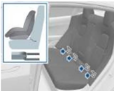
Once installed, test the security of the installation before seating a child. Attempt to twist the child safety seat from side to side and try to pull it away from the seat, then check to ensure the anchors remain securely in place.
