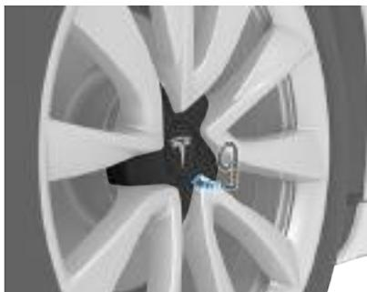
2. Maneuver the lug nut cover tool so that it is fully inserted into the hole in the lug nut cover.
