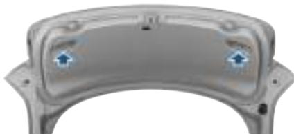
**Warning:** Before driving, ensure that the trunk is securely latched in the fully-closed position by lifting up on the bottom edge and confirming there is no movement.
