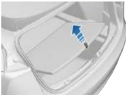
**Caution:** Never load more than 130 lbs (60 kg) on the rear load floor (above the lower trunk compartment) or more than 285 lbs (130 kg) in the lower trunk compartment. Doing so can cause damage.
