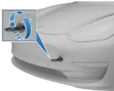
5. Attach the winch cable to the tow eye.
