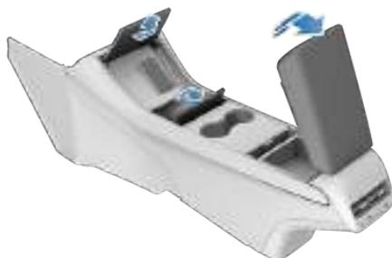
To open the main storage compartment, pull its cover upward.
