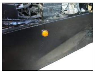
The high stop light is fitted by cutting a rectangular hole that is 220mm x 20mm and 60mm from the top of the panel and in the centre of the panel. The high stop light is then fitted in the hole and held in place by two self tapping screws
