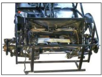
The rear shock absorbers are attached to the rear wishbone and to the bracket on the chassis. The top mount is held with a 1/2" UNF bolt and the bottom shock mount needs a 12mm sleeve fitted as the MX5 has a M12 bolt. Use spacers to ensure clearance between the spring and the half shaft.
