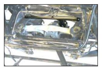
The crossbar is placed on top of the frame and bolted to the **U** bracket.
