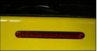
The number plate light is fitted in the centre of the panel approximately 240mm from the bottom edge.
