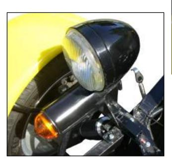
The indicator is fitted to the front of the cover and the wires plus the headlight wires with a sleeve are fitted and fed through the hole in the side of the bracket and through the square tube.
