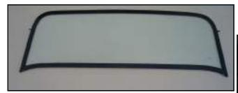
Using a black sealant, attach the lower lip of the windscreen frame.
