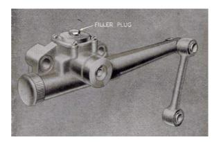
Fig. 47 Type P.R.6/ 12 Shock Absorber
