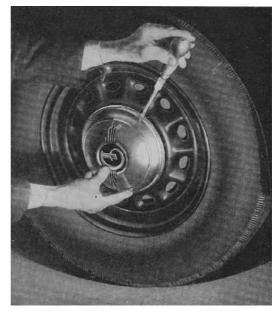
Fig. 36 Removal of Hub Cover Plate
