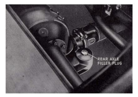
Fig. 34 Rear Axle Filler and Level Plug ("Special Sports")
