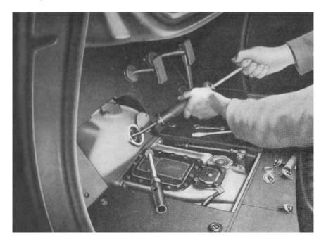
Fig. 28 Topping up The Fluid Flywheel
