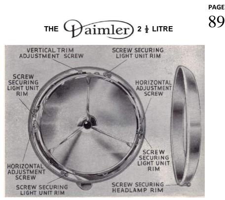
Fig. 47 Headlamp with Front Rim removed
