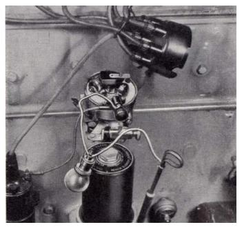
Fig. 26 Setting Ignition Timing.
