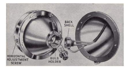
Fig. 48 Headlamp with Light Unit removed
