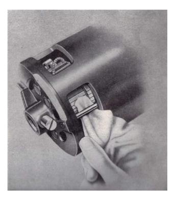
Fig. 51 Cleaning Commutator
