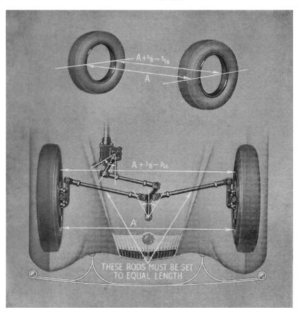
Fig. 43 The Setting of the Front Wheel Alignment
