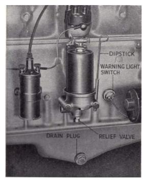
Fig. 16 Location of the Sump Drain Plug and Dipstick
