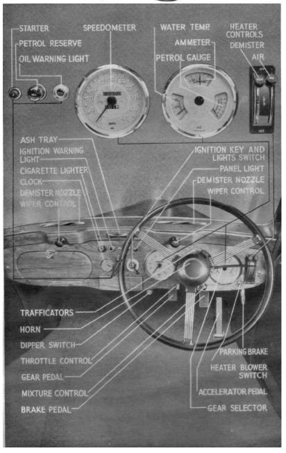
Fig 1 The Controls and Instruments ("Consort" Saloon)
