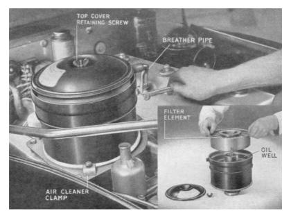
Fig. 11 The Oil Bath Air Cleaner and Silencer ("Special Sports")
