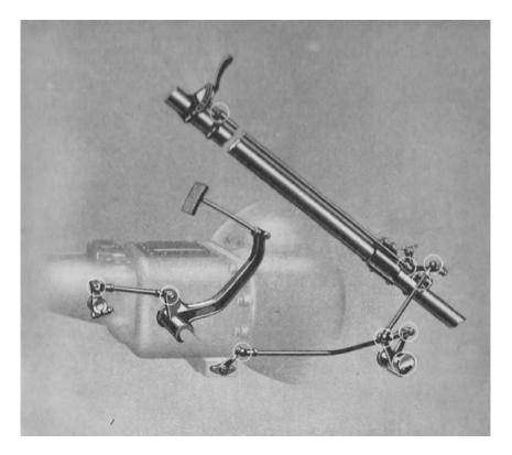
Fig. 30 Gearbox Control Rods Lubricate with oil can where indicated by rings
