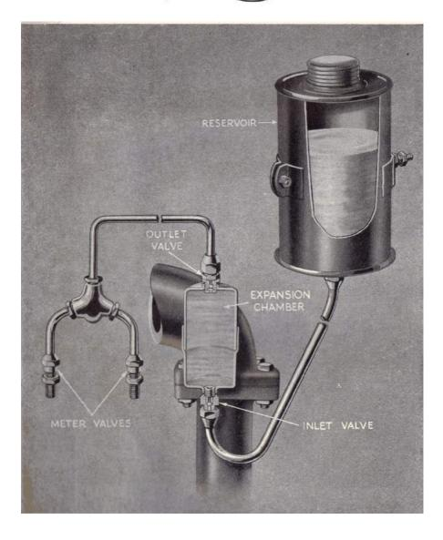
Fig. 60 Chassis Lubrication Operating Mechanism
