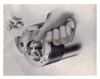
Fig. 52 Cleaning Commutator
