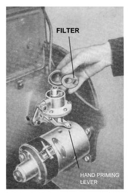
Fig. 12 The Petrol Pump Filter and Hand Priming Lever
