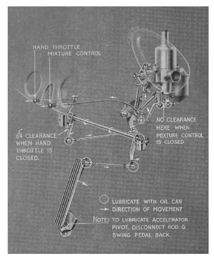
Fig. 10 The Carburettor Controls ("Consort" Saloon)
