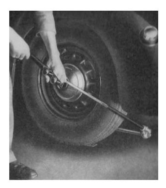
Fig. 62 Operating one of the two Rear Jacks
