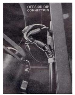
Fig. 46 Headlamp Wiring Connections
