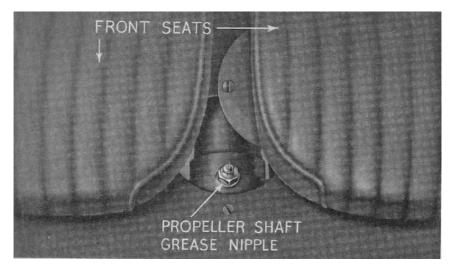
Fig. 33 Propeller Shaft, showing the Grease Nipple
