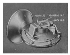
Slacken the locknut on the fixed contact and rotate the adjusting nut until the contacts are just separated (indicated by horns failing to sound). Turn the adjusting nut half a turn in the opposite direction and secure in this position by tightening the locknut. Finally, if the note is still unsatisfactory, do not dismantle the horn, but return it for examination.
