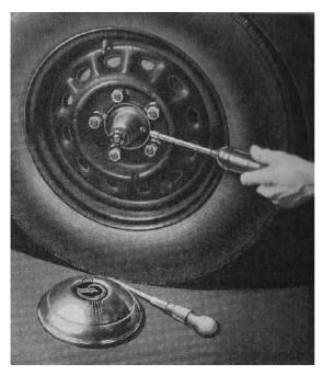
Fig. 38 Rear Hub Grease Nipple
