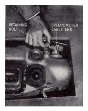
Fig. 32 Speedometer Cable
