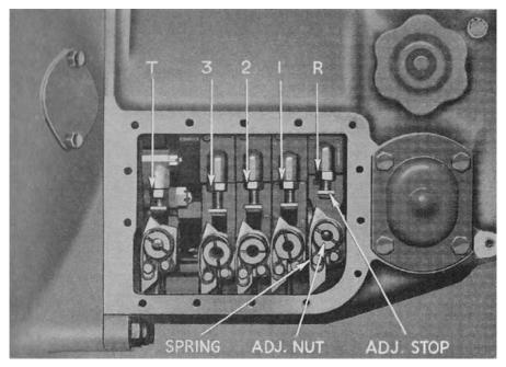
Fig. 31 Adjustment of Toggle Setting
