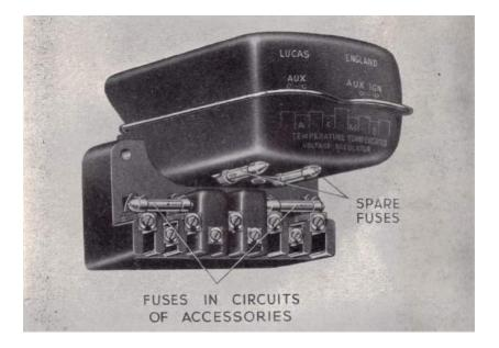
Fig. 55 Control Box and Fuse Box
