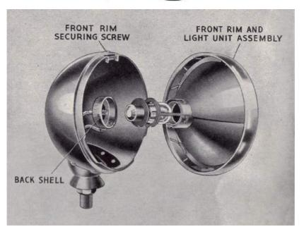
Fig. 49 Headlamp with Light Unit removed
