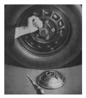
Fig. 37 Removal of Hub Cap (Front Wheel)
