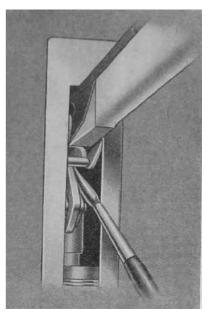
Fig. 57 Lubricating Trafficator
