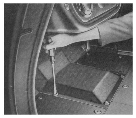
Fig. 27 Removing Fluid Flywheel and Gearbox Cover
