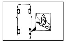
After the vehicle is lifted by the jack, it is necessary to place tire stops in the front and rear side of the tire diagonal to the ruptured tire to prevent it from rotating.
