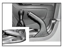
After parking the vehicle, you must use hand brake. When the ignition key is in "ON" or "START" position, hand brake indicator will illuminate. Before driving, you must release hand brake and confirm if the indicator extinguishes.
