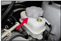
To service the engine hood, it is necessary to inspect the clutch liquid level of the general braking pump. The system should also be checked for possible oil leakage. Check and confirm that the clutch level is between "MAX" and "MIN". Add a suitable amount of clutch liquid as required. Decrease of level means leakage existing in the clutch system, and a timely inspection should be made to identify the leaking position and have it repaired. Consult your JAC dealer for detailed repair
