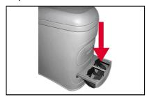
In order to fix water cup or drink tin, the cup holder in rear seat is installed on the main console of rear seat. You can use it by pressing the top of the cup holder.
