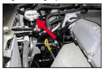
Use an ethylene or ethylene glycol cooling liquid with water at a mixture ratio of 50/50. The engine cooling liquid should be compatible with the parts of aluminum alloy engine. Never use additional inhibitor or additive. The cooling system should used engine cooling liquid with correct concentration and anti-freezing and anti-corrosion performance.
