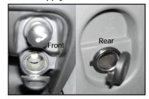
These sockets can supply power of 12V voltage. Thus, all kinds of electrical accessories and equipment can be run.
