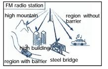
FM radio receives high frequency signals that can not bend with the earth curvature. So, FM radio can only receive signal which is near to service station. In the same way, FM signal will be influenced by high building, high mounting or other barrier. These reasons may lead to unclear sound. The following phenomena are normal; do not regard them as radio's malfunction.
