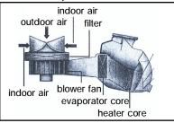
Air conditioner is inside of the evaporator, which is back of the glove box. This unit can reduce foreign materials that come into vehicle and filter with air.
