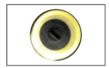
When the door is open, the ignition switch will illuminate to inform you that the ignition switch is not in "ON' position. When the door or the igni-
