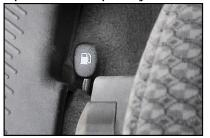
Pull up the release rod (on the floor) in the left front corner of driver seat and open the filler cap.
