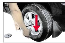
To fit the wheel cover again, place the nuts on studs and tighten them. Swing the wheel gently to confirm if it has been safely fixed, and tighten the nuts with hands again.
