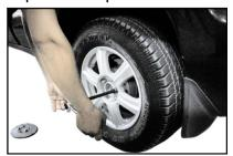
The following is about replacement of a ruptured tire. When it is necessary to replace a ruptured tire, confirm that the transmission is set to the reverse gear (manual transmission), and the parking brake is applied. After that:
