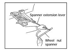
Fit the jack handle at the position shown. To raise the vehicle, turn the handle clockwise. Confirm the position of the jack when jacking the vehicle to avoid it sliding down. If the jack is placed on a soft ground or beach, a suitable plate is needed and should be placed at the bottom of the jack, to avoid loss of balance. Raise the vehicle sufficiently high to allow mounting the spare tire.
