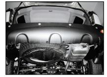
Remove the spare tire and take out the jack, jack handle and tool bag.
