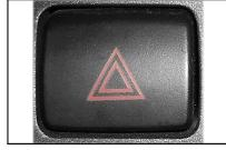
If you need to brake for emergency in a dangerous place, you should use hazard warning system. For such braking, please select appropriate position.
