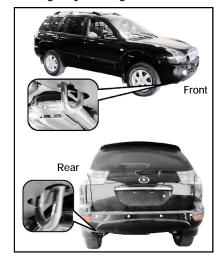
If no professional towing vehicle is available, tie the towing cable chain or lifting lever on the bottom hook at the front of the vehicle, and tow the vehicle in emergency. Operate with
