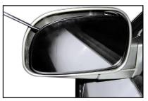
Pushing the mirror towards vehicle can fold the mirror. By that way, the vehicle can be parked in narrow place
