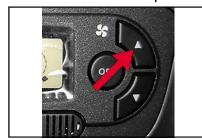
Pressing control button for fan speed can set the fan speed to appropriate value. Faster speed can provide higher air flow. Pressing "OFF" button can close the fan.
