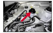
The power steering oil level should be inspected periodically. To check the power steering oil level, turn off the ignition switch and check the power steering oil tank level. This level should be between "MAX" and " MIN".
