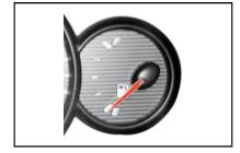
Fuel gauge indicates the fuel level in the fuel tank.
