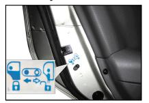
Your vehicle is equipped with child safety lock in rear door. You should lock the rear door, to ensure that it can not be opened from inside. This manual recommends using this device with child in the rear seat.
