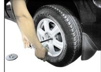
Replace a tire with one of the specified size. And for tire replacement, refer to the JAC Instruction Manual about wheel rim grooves and adjusting deviations.
