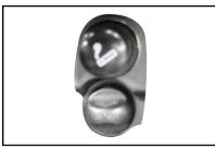
To use the cigarette lighter, press and then release it immediately. When it becomes hot, it will jump up automatically, and then you can use it. If the engine is not started, the cigarette lighter can not be used unless the ignition switch is in "ACC" position. To avoid damaging the socket or fire, do not use counterfeit accessories.
