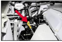
Before check the engine oil, warm up the engine to normal water temperature and park the vehicle on a flat ground. Turn off the engine and wait for several minutes. Pull out the oil stick, wipe off the oil, and insert the oil stick again and then pull it out again. Record the final oil level on the stick. The level should be between the full ("F") and low ("L") positions.
