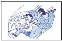
Safety belt pretensioned belt is installed in the driver seat and front seat. The aim is to protect the driver and the passenger in the front seat in case of serious impact. In such case, the pretensioned safety belt in the front seat and the air bag will operate at the same time.
