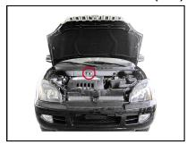
You may use the VIC to register your vehicle and handle legal affairs about it. The VIC is located in the vehicle identification code panel of the fire wall between the engine and driver cab.
