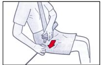
Tie the safety belt, pull out safety belt tongue from expansion box and insert into the snap ring until you hear a "ka" sound.
