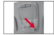
Press the reading light switch to turn it on or off. The reading light can be used to light in night or be used as private light of the driver or passenger.
