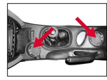
In order to take out the water cup or drink tin easily, the cup holder is installed on the main console.
