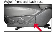
Incline forward a little, and pull backward the link which is near the seat. Incline the seat backward and adjust to the desired position. After positioning, undo the link.
