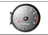
The tachometer indicates engine speed. Use the tachometer to select correct gear, avoiding use low gear or high gear at low speed.
