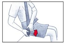
Press down the loosening button on the buckle. After being undone, the safety belt will return to expansion box automatically.
