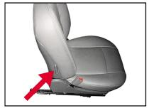
Adjusting the seat back control, in order to increase weight of seat back, put the adjusting rod to rear position.
