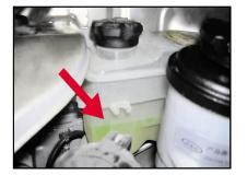
Replace engine cooling liquid Replace engine cooling liquid as per the maintenance schedule.
