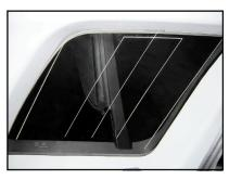
When the ignition key is in "ON" or "ACC" position, if you turn on the radio, the vehicle will receive AM and FM signals from rear side glass.
