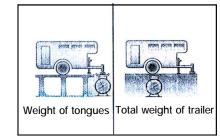
The weight of the trailer is adjusted by adding or reducing the number of tongues. Check the total weight of the trailer and the weight of the tongues.
