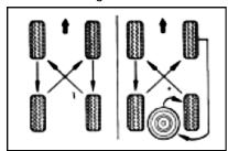
Wheel shifting shall be performed every 10,000km. If uneven wearing is found after shifting, have the JAC dealer check the vehicle for timely correction.
