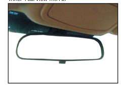
The inner back mirror can be adjusted upward, downward, leftward and rightward. Adjust the daily and night vision of the mirror by using the inner rearview mirror adjust rod. This adjustment will reduce the glare of the headlight at the back of your car.
