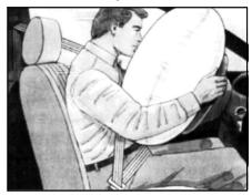
The driver airbag locates on the center of the steering wheel.
