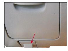
1. Pull the engine cover release bar at left lower side of console.
