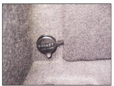
Your vehicle is equipped with an accessory power supply socket. You can connect the accessory electrical equipment through accessory power supply socket. The accessory power supply socket is in the trunk. To use the power supply socket, remove the protective cover first. When the socket is not used, make sure to close the protective cover. The
