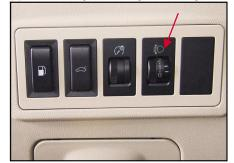
The fourth switch on the left switch group assembly on the instrument desk is the dimming switch of headlight which could adjust the illumination angle of the dipped beam light and high beam light. Toggle the thumbwheel switch of the dimming switch upward to upper the beam of dipped beam light and high beam light and vice versa.
