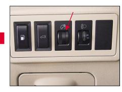
The third switch on the left switch group assembly of instrument desk is the dimming switch which can adjust the brightness of the light on the console.
