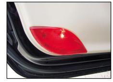
When you open the front door or rear door, the door control lamp inside the vehicle will be on. The door control lamp is located at inside of driver and front passenger door and rear passenger door. When you close all the doors, this lamp will be off.
