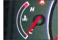
Indicating the water temperature of the engine. When the pointer reaches the red area, the car must be stopped for overhaul, preventing the engine damage. It should not be restarted until the water temperature decreases. If such similar fault still exists, please promptly contact with the special service center of Jianghuai Automobile Company.
