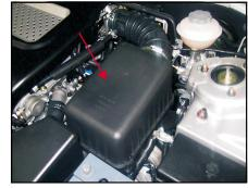
According to the maintenance regulation introduced in this manual, check and replace air filter element regularly.
