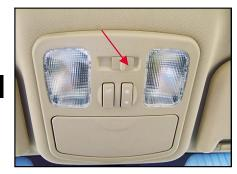
The front dome lamp and rear dome lamp switches have three positions. ON position will switch on the dome lamp. The dome lamp will keep being on until it's switched off manually. When the switch is turned to middle position, the dome lamp will be switched on upon opening of any door. When the door is
