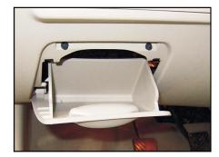
The storage box at driver's side locates at the console at the left side of steering wheel. It is used as the interior fuse check mouth as well. To use it, just pull out the storage box or take it out.
