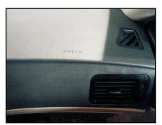
Your vehicle has been equipped with two airbags, one is the frontal airbag for the driver, and the other one is the frontal airbag for the right front passenger.
