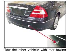
hook. The rear towing hook can be used in emergency only (for example, tow the vehicle trapped in the ravine, snow or slough).
