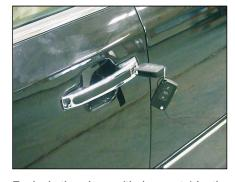
To lock the door with key outside the car, you should insert the key and turn it clockwise.
