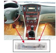
It's located at the driver and copilot feet position for feet lighting.
