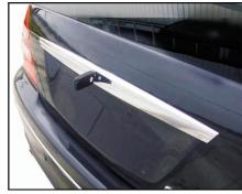
To open the boot cover, please insert the key and screw it clockwise, lift the boot cover and return the key to neutral position and then pull it out. To close the cover, please press the boot cover downward and lock it.
