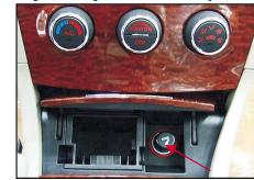
The front cigarette lighter and ash tray locate at the lower part of the central console with an integrated protective cover. Press at the bright stripe ornament part on the cover and then release, the protective cover will open automatically. To take out the front ash tray for cleaning, pull out the ash tray and pour the ash. When reassembling, just push the ash tray back.
