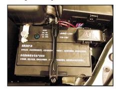
There is maintenance free storage battery installed in your vehicle. If you want to replace the storage battery, the part number on volume of all the storage battery shall be the same with that of the original storage battery. See "General Drawing of Engine Cabin" in this section to confirm the position of the storage battery.
