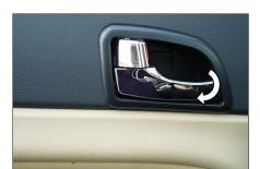
To open the door from inside of the car, pull the door handle inwards.
