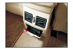
The rear ash tray locates at the rear part of auxiliary facia console. Pull out the rear ash tray for cleaning. When reassembling, just first clamp it on the bottom tongue and then push it back.
