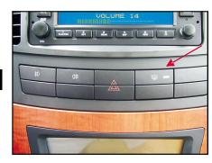
Your vehicle is equipped with a rear window and exterior view mirror defroster, which can operate only when the ignition switch is switched on.
