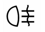
When the front fog lamp is on, press the rear fog lamp button on the mid switch group assembly of instrument desk, the front fog lamp will be connected and the rear fog lamp indicator light on the combined device will light on. The indicator light on the button will light on.
