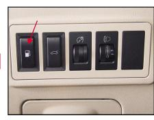
Press the oil tank cover switch on the left switch group assembly of instrument desk, and you can open the oil tank cover.
