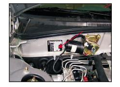
3. Body VIN code under the engine hood This VIN frottage is not on the nameplate, but carved on the body under the engine hood and above the nameplate.
