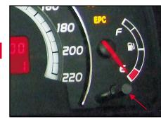
The reset lever can be used to shift among modes, adjust time and reset the odometer. When operating the shift display modes, one must press it in short time (>300ms and <2s).
