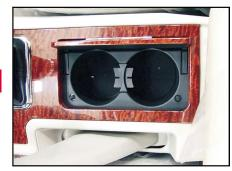
The cup support locates at the auxiliary facia console and rear seat armrest. To use the front cup support, press the bright stripe ornament part of the cup protective cover and then loosen, the cover will open automatically. To use the rear cup support, pull down the central handle at rear seat (refer to the next page "Rear Seat Armrest".
