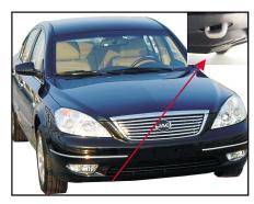
The front towing hole is located under the front guard. There shall be a driver in the vehicle to control steering and braking.
