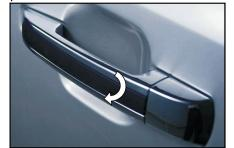
To open the door from outside of the car, pull up the door handle outwards.
