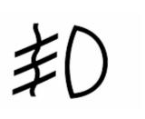
Press the front fog lamp button on the mid switch group assembly of instrument desk, the front fog lamp will be connected and the indicator light on the button will light on. At the same time, the front fog lamp indicator light on the combined device will light on. Press the button once again and the front fog lamp will distinguish.
