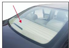
It's located at the rear window defroster and equipped with AM-FM antenna. Ensure there is no scratch on the internal surface of rear window and the grid line on the rear windscreen is not damaged. If the internal surface of rear window is damaged, it may interfere with radio receiving signal. In addition, to ensure normal receiving signal of radio, the antenna signal amplifier in rear right C pil-
