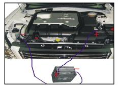
Connect the jumper cable according to the following sequences when starting the vehicle:
