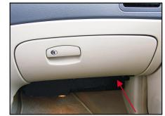
The glove compartment is equipped with locking core. You can lock and unlock the glove compartment by the ignition key. To open the glove compartment, just pull upward the glove compartment handle when the compartment is at unlocking position.
