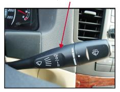
Operate the front windshield wiper by using the control lever at the right side of the steering column. The ignition switch must be connected to operate the wiper. Clearance: turn the handle downward to the 1st shift and select one cycle of delayed wiping and washing.
