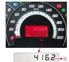
With accumulated mileage, mileage subtotal and time showing function
