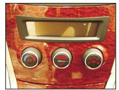
AUTO (automatic): press AUTO button to enable automatic control over internal air temperature, air delivery mode and fan speed. Then, the AUTO mode indicator will present on the display.
