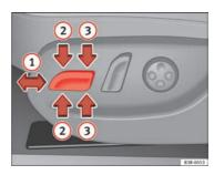
Fig. 106 Front seat: Seat adjustment switches
