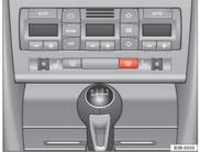
Fig. 96 Switch for heated rear window
