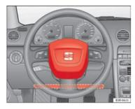
Fig. 18 Driver airbag in the steering wheel and knee airbag in the dash panel
