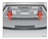
Fig. 35 Position of the Top Tether rings on the rear tray
