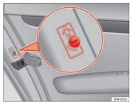
Fig. 77 Childproof lock on the rear doors
