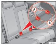
Fig. 33 Position of the ISOFIX anchors on the side rear seat
