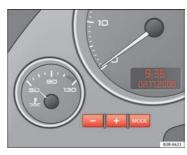
Fig. 41 Detailed view of the instrument panel: Digital clock
