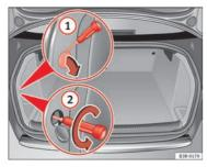
Fig. 210 Luggage compartment: Location of the bolt securing the tail light unit
