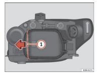
Fig. 201 Side light bulb (inside of vehicle)
