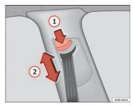
Fig. 17 Belt height adjuster
