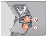
Fig. 221 Position of the bulbs in the bulb holder Example: Tail lights on the rear lid
