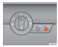
Fig. 85 Detailed view of the dash panel: Coming home and leaving home functions
