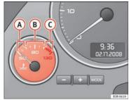
Fig. 39 Engine coolant temperature gauge
