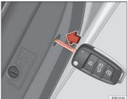
Fig. 74 Activating manual locking
