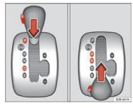
Fig. 149 Selector lever lock
