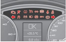
Fig. 45 Instrument panel with warning and indicator lamps
