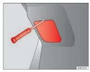
Fig. 219 Remove the cover from the rear lid
