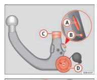
Fig. 157 Removable towing bracket: Ball joint
