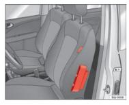
Fig. 24 Side airbag in driver seat
