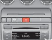
Fig. 90 Centre console: Switch for hazard warning lights
