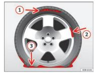
Fig. 187 The Tyre Mobility System is not suitable for repairing this type of damage to tyres.
