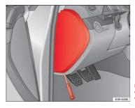
Fig. 189 Fuse box cover on the left side of the dash panel.
