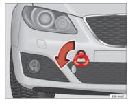
Fig. 232 Fitting the towline anchorage to front of the vehicle
