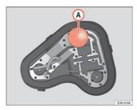
Fig. 214 Position of the bulb on the bulb holder. Example: Left tail light in side panel.
