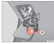
Fig. 222 Position of the bulb on the bulb holder. Example: Tail lights on the rear lid
