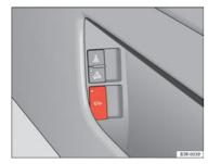
Fig. 75 Driver door: Unlocking the rear lid
