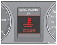
Fig. 55 Display: Coolant level warning
