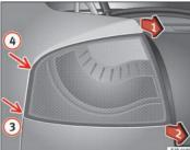
Fig. 211 Remove rear light unit from side panel
