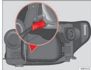
Fig. 202 Side lights. Bulb holder grip in vertical position
