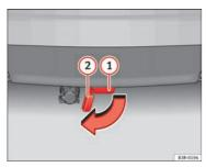
Fig. 156 Rear bumper: Open the cover piece
