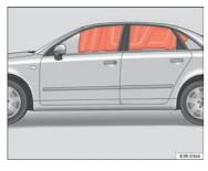
Fig. 27 Deployed curtain airbags
