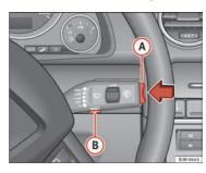
Fig. 61 Windscreen wiper lever: Onboard computer controls
