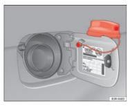
Fig. 167 Fuel tank flap with tank cap attached
