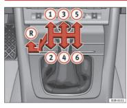
Fig. 146 Detailed view of the centre console: gear shift pattern of a 6-speed manual gearbox
