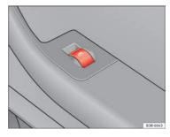
Fig. 81 Switch on front passenger door
