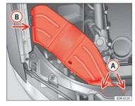
Fig. 203 Air duct on right side of vehicle
