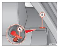
Fig. 115 Backrest release lever
