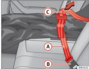
Fig. 117 Securing the ski bag on the centre seat belt buckle on the rear seat bench
