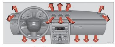
Fig. 131 Dash panel: Location of air outlets
