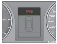
Fig. 46 Display: system fault
