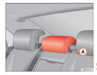
Fig. 112 Centre rear seat: Head restraints
