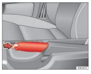
Fig. 142 Detailed view of the centre console: Handbrake on
