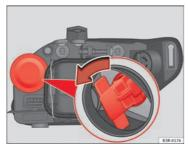
Fig. 207 Turn signal bulb
