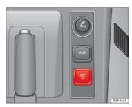
Fig. 177 Detailed view of the centre console: Button for the tyre pressure monitoring system
