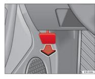
Fig. 168 Detail of footwell area on driver side: lever for unlocking the
