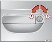
Fig. 71 Turning the key to enable the open and close functions
