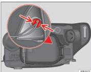
Fig. 200 Side light bulb (outside of vehicle)
