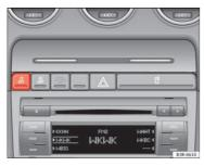
Fig. 153 Centre console with ESC switch
