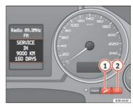
Fig. 53 Detailed view of the instrument panel: Service indicator
