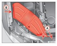
Fig. 192 Air duct on right side of vehicle
