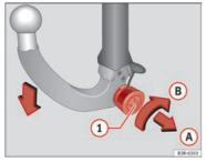
Fig. 163 Removable towing bracket: Removing the ball joint
