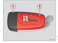
Fig. 70 Master key: Opening the cover
