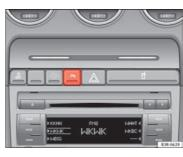
Fig. 143 Centre console: switch for parking aid
