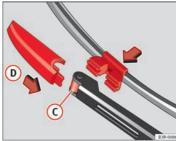
Fig. 175 Fitting the wiper blade
