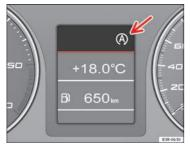
Fig. 139 Display on the instrument panel during Start-Stop function oper-
