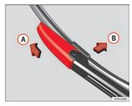
Fig. 174 Removing the wiper blade
