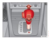
Fig. 150 Centre console: Manual gear selection (tiptronic mode)
