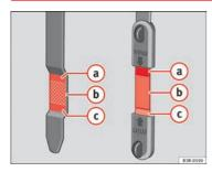
Fig. 170 Markings on oil dipstick
