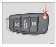
Fig. 68 Remote control key: Release button
