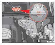
Fig. 176 Engine compartment: markings on brake fluid reservoir
