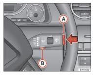
Fig. 64 Windscreen wiper lever: Reset button and rocker switch
