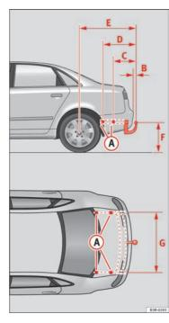
Fig. 165 Attachment points for towing bracket
