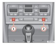
Fig. 132 Detailed view of the dash panel: Thumbwheel controls for seat heating
