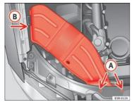
Fig. 204 Air duct on right side of vehicle
