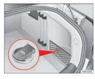
Fig. 124 Detailed view of the side trim in the luggage compartment: 12 volt power socket
