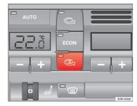
Fig. 130 Button for automatic air recirculation
