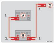
Fig. 230 Diagram of connections for vehicles without Start Stop system
