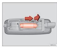
Fig. 229 Removing sun visor light
