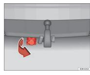
Fig. 162 Rear bumper: Pulling down the power socket
