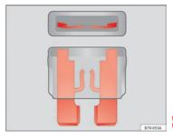
Fig. 190 Image of a blown fuse
