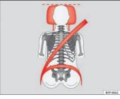
Fig. 13 Correct seat belt and head restraint positions, viewed from front
