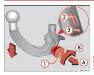
Fig. 159 Removable towing bracket: Setting the spring mechanism to the "ready" position
