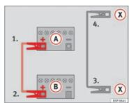
Fig. 231 Diagram of connections for vehicles with Start Stop system
