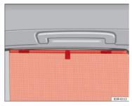
Fig. 98 Sun blind extended to cover rear side window
