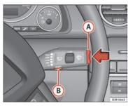
Fig. 59 Windscreen wiper lever: Function selector switch
