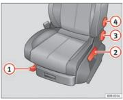
Fig. 104 Adjuster controls on driver seat
