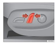
Fig. 107 Front seat: Backrest adjuster switch
