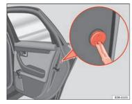
Fig. 73 Manual locking device
