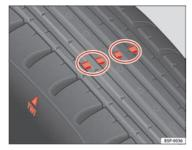
Fig. 178 Tyre tread wear indicators
