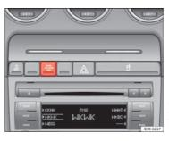
Fig. 29 Control lamp for deactivated front passenger airbag in centre console
