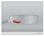
Fig. 228 Removing sun visor light
