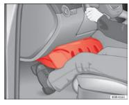
Fig. 23 Inflated airbags protect in a frontal collision.
