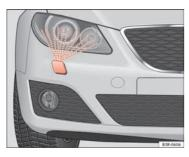
Fig. 101 Headlight with extended washer jet
