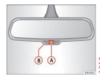
Fig. 102 Interior mirror with anti-dazzle setting: Indicator lamp and on/off switch
