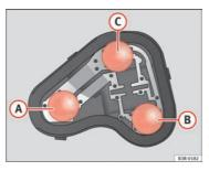
Fig. 213 Position of the bulbs in the bulb holder Example: Left tail light in side panel.
