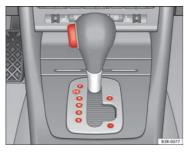
Fig. 147 Detailed view of the centre console: Selector lever with lock but-
