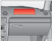
Fig. 19 Front passenger airbag located in dash panel
