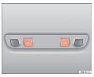
Fig. 94 Detail of headliner: rear reading lights
