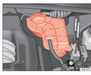
Fig. 172 Engine compartment: Coolant fluid deposit
