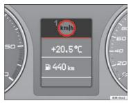
Fig. 57 Display: Speed warning function
