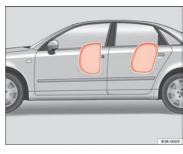
Fig. 25 Inflated side airbag on left side of vehicle
