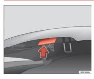
Fig. 169 Release catch under the bonnet
