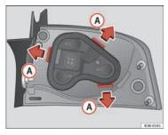
Fig. 212 Retaining tabs on reverse side of tail light
