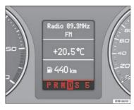
Fig. 148 Display: Selector lever positions
