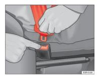
Fig. 16 Remove latch plate from buckle
