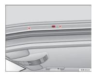
Fig. 118 Attachment points for basic support units
