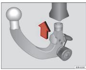
Fig. 160 Removable towing bracket: Inserting the ball joint
