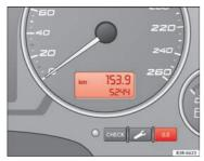
Fig. 43 Detailed view of the instrument panel: Odometer
