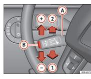
Fig. 144 Controls for the cruise control system
