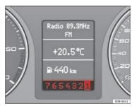
Fig. 151 Display: Manual gear selection (tiptronic mode)
