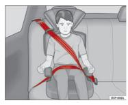
Fig. 32 Forward-facing child seat installed on rear seat
