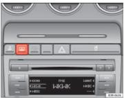
Fig. 99 Switch for electric sun blind on rear window
