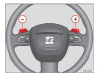
Fig. 152 Steering wheel: tiptronic controls
