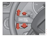
Fig. 91 Turn signal and main beam headlight lev-
