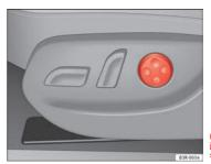
Fig. 108 Front seat: Adjuster switch for lumbar support
