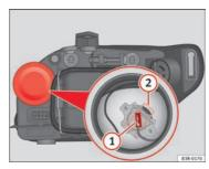
Fig. 196 Main beam headlights
