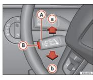
Fig. 145 Controls for the cruise control system
