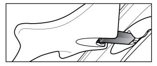
(B) Open the boot compartment. Pull the handle upwards to disengage the roof securing pins.
