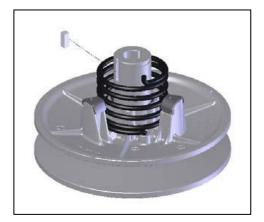
Position the spring (4) in the sliding flange (2) at the position noted during removal.
