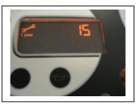
If the mileage remaining before maintenance exceeds 200 km and the time remaining is less than 20 days, the LCD displays the number of days flashing + the « key » symbol + the « 1 year » symbol for 5 seconds.
