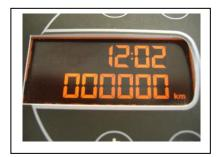
If the sensor is not connected (circuit open) or if the sensor is in short-circuit, there is no display.
