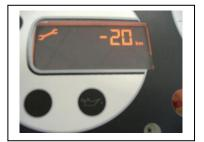
If the total mileage before maintenance has been exceeded, the LCD displays the mileage in negative flashing + the « key » symbol for 5 seconds.
