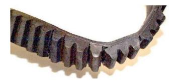
> Change the belt when it reaches a width of 28.5 mm, i.e. about 2 mm narrower than the new belt.
