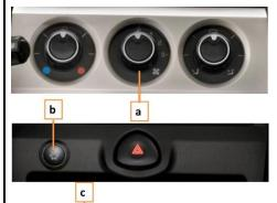
a/ Fan speed controlerb/ A/C commutatorc/ Air recirculation speed
