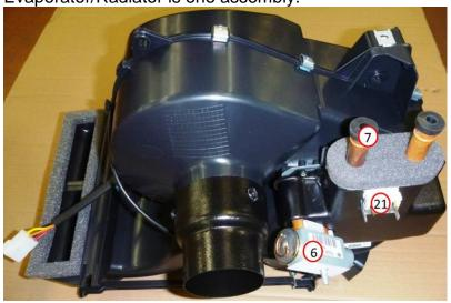
6 TXV - 5 HP Service Port - 8 LP Service Port: The ports are behind the dashboard, passenger side.
