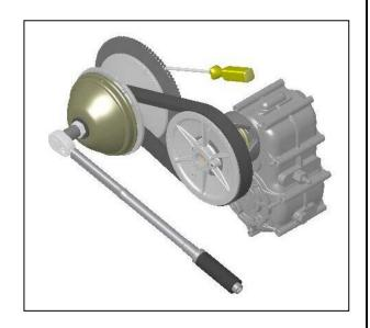
Do not forget to remove the opening screw from the led pulley flask. Otherwise, the pulley could be unbalanced.
