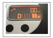
If the mileage for maintenance is exceeded, the LCD displays the « key » symbol on the left-hand display, permanently.
