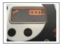
If the mileage exceeds 200 km before maintenance, the LCD displays the mileage remaining + the « key » symbol for 5 seconds.
