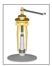
Using a puller is required to prevent damaging the parts which do not require changing.
