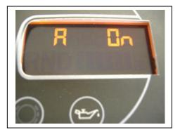
This message means the automatic warning lights function is activated.
