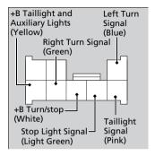
Your trailer lighting connector is located under the right side tool case in the cargo area. Each pin's purpose and wiring color code are shown in the image.
