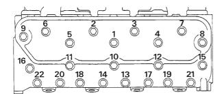
Fig.6 Head bolt tightening sequence
