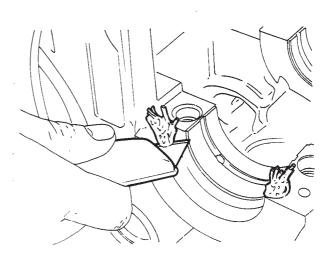
Fig.3 Trimming seal ends
