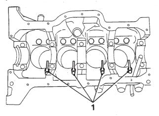
Fig.2 Piston oil jets (ET engine only)
