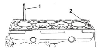
Fig 5 Fitting cylinder head
