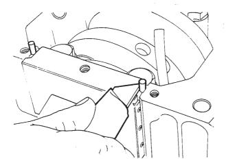
Fig.6 Trimming rubber seals
