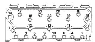
Fig.1 Cylinder head bolt slackening sequence
