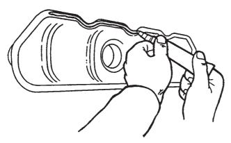
Fig.1 Applying silicone sealant
