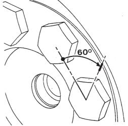
Fig.3 Flywheel bolt tightening sequence
