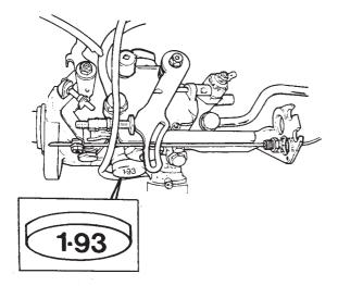
Fig.12 Fuel injection pump timing setting
