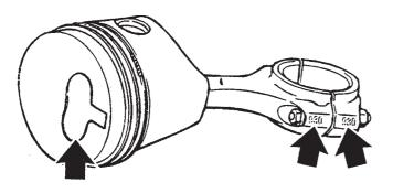
Fig.6 Fitting piston to connecting rod
