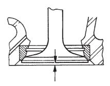
Fig.3 Valve recession
