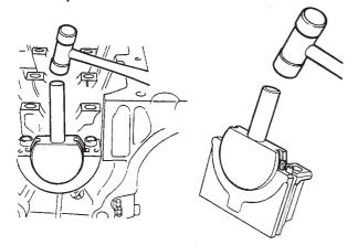
Fig.2 Shaping the seals with tool 0480061
