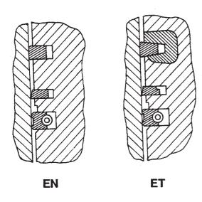
Fig.4 Piston ring layout
