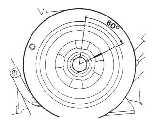
Fig.3 Tightening crankshaft pulley nut
