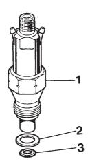
Fig.11 Injector and sealing washers
