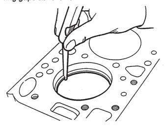
Fig.5 Measuring ring gap
