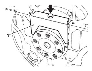
Fig.5 Using tool 0480062 to fit bearing cap
