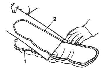
Fig.2 Fitting rocker cover cord gasket
