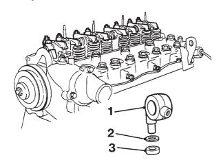
Fig.9 Rocker shaft oil supply union
