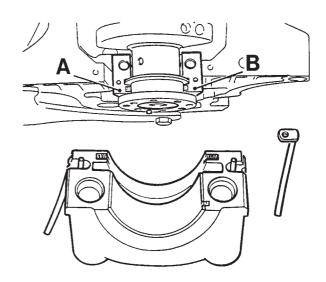
Fig.4 Rear main bearing cap rubber seals
