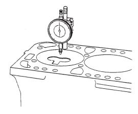
Fig.3 Measuring piston protrusion
