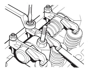
Fig.10 Adjusting valve clearances
