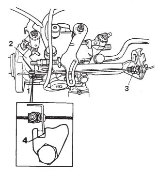
Fig.12 Fast idle cable
