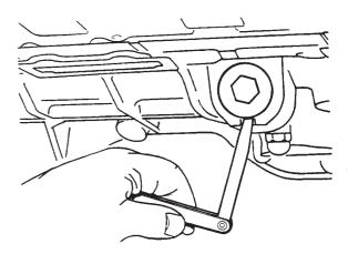
Fig.4 Measuring thrust cap gap
