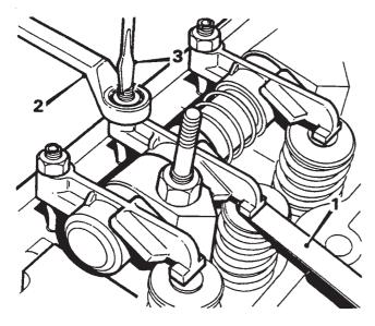
Fig.1 Rocker adjustment
