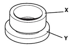
Fig.2 Machining swirl chamber to adjust protrusion
