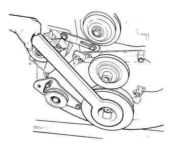
Fig.1 Holding crankshaft with 0480060
