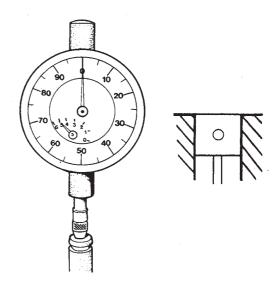
Fig.5 Piston gauge reading - stage 1
