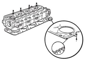
Fig.2 Selecting cylinder head gasket
