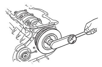
Fig.1 Measuring crankshaft torque-toturn.
