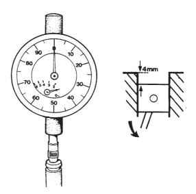
Fig.6 Piston gauge reading - stage 2
