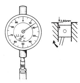
Fig.7 Piston gauge reading - stage 3
