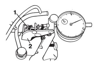
Fig.9 Fitting tool 0480066 & dial gauge
