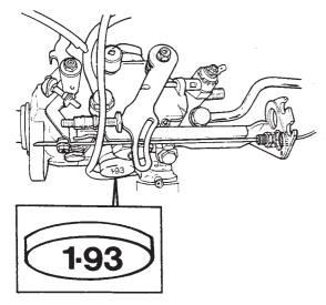
Fig.1 Fuel injection pump timing setting
