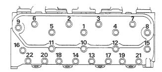
Fig.13 Cylinder head tightening
