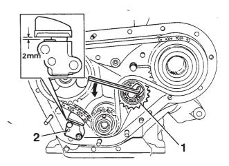
Fig.10 Tensioning chain
