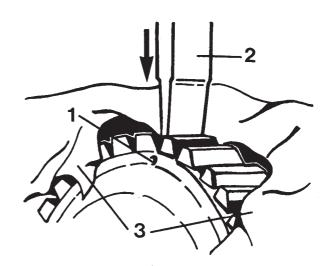
Fig.2 Removing starter ring gear
