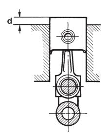
Fig.4 Piston protrusion
