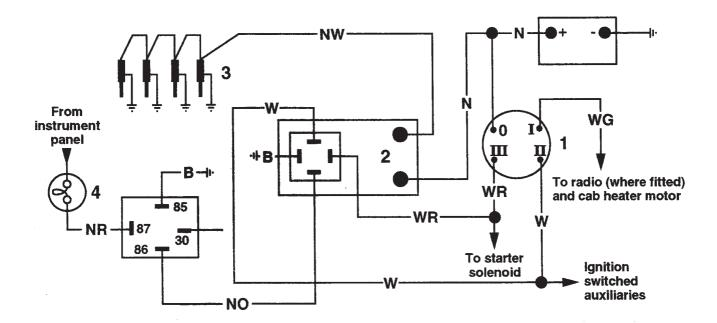
Fig.1 Heater plug circuit
