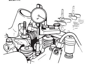
Fig.4 Dial gauge on No.7 valve
