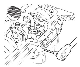
Fig.2 Fitting oil pump
