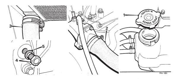
Fig.1 Coolant drain and refill
