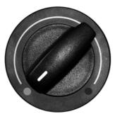
The air temperature in the car can be controlled by operating the temperature control knob (B) on the control panel. The temperature can be increased by rotating the knob towards the red segment and decreased by rotating it towards the blue segment. (C) Blower Speed Regulation Knob:
