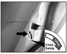
Both the rear doors of the car are provided with a child proof lock. Push the lock lever located on vertical face of the door near the lock downward before closing the door. The door which has been locked by activating the child lock cannot be opened from inside, it can be opened only from the outside.
