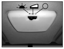
Interior roof lighting and reading lamps with inbuilt switches are provided on the roof near the rear view mirror.
