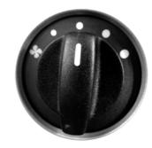
The HVAC system has a four speed blower. The blower speeds can be regulated by operating the blower knob (C) at the centre of the control panel.
