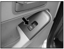
Window Winding Switch on Rear Door
