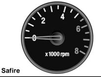
engine rpm unneccessarly, The permitted engine rpm upper limit is the start of coloured zone on the dial.
