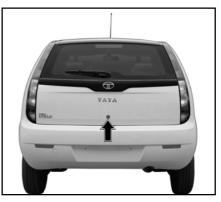
It can also be opened by using door key. The lock is located on the trunk lid.
