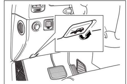
2. Press the safety catch lever up located under the front edge of the hood and lift the hood fully.
