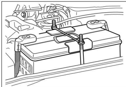
Check the battery terminals for corrosion (a white or bluish powder). To remove it, cover the terminals with a solution of baking soda and water. It will bubble up and turn brown. When this stops, wash it off with plain water. Dry off the battery with a cloth or paper towel.
