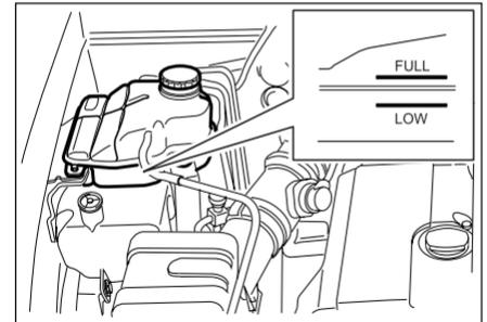
In order to protect your vehicle in extremely cold weather, use a mix 40% distilled water and 60% antifreeze specified.
