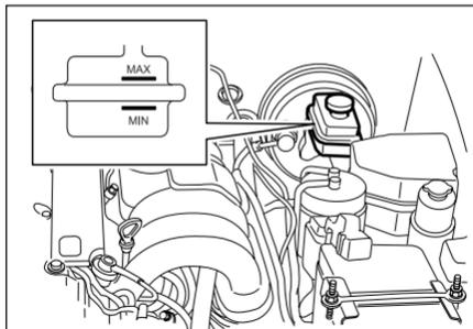
To add the brake fluid, first wipe away dirt and then unscrew the fluid tank cap. After removing the cap, top up the fluid to the MAX mark and tighten the cap securely afterwards.
