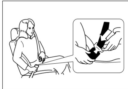
To remove the belt, depress the red push-button on the buckle. The belt will retract automatically.
