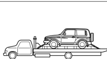
Your vehicle (4 Wheel Drive Vehicles) should be towed with towing dolly under the wheels or on a flat bed.
