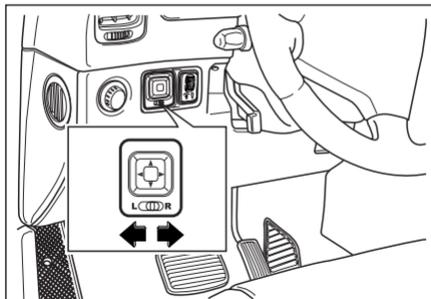
1. Select the mirror you want to adjust by using the left/right switch, located just below the mirror adjustment pad, to the left for left mirror or to the right for right mirror.
