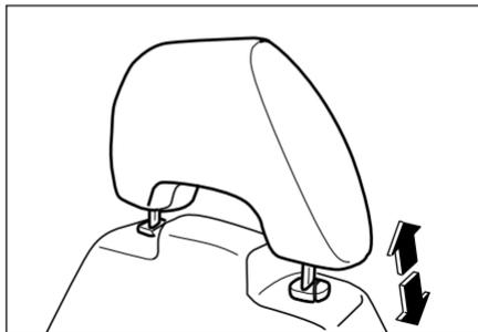
To remove the head restraint
