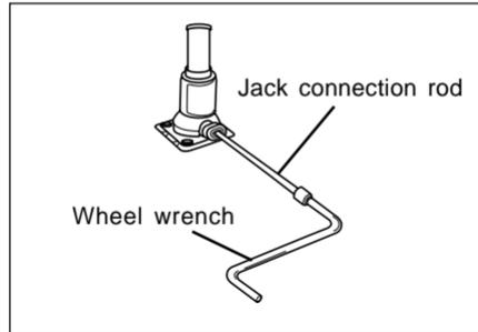
6. Place the jack vertically at the front or rear jacking location closest to the wheel you plan to change.
