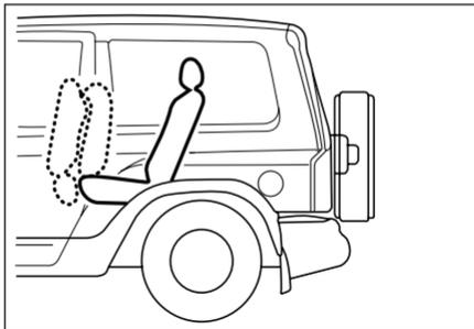
8. Make sure the seat belts are not twisted or caught in the seatback and are arranged in their proper position.
