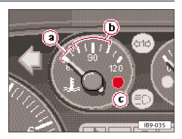
If the needle is in the right half of the indicator, the coolant temperature is too high. In this case, pull over, switch the engine off, wait until it cools and then look for the cause of the problem. See the chapter on "Cooling system".
