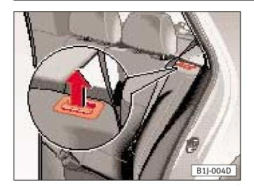
• Pull the release lever on the backrest in the direction of the arrow (or both levers at the same time if the seat is not split) and lower the backrest.
