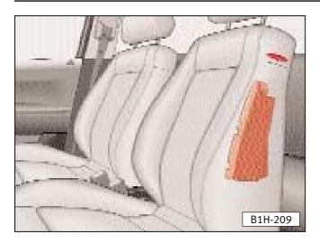
The **side Air Bags** are located on the backside of the front seats (see figure) and are marked with "AIR BAG" on the upper part of the back.
