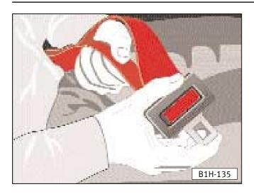
**To lengthen** belt hold the tongue at right angles to belt and pull belt through to the required length – see illustrations.
