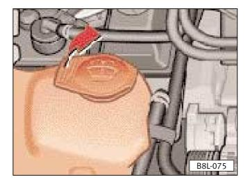
The fluid container is on the right of the engine compartment. The container holds about 3 litres: on vehicles with a headlight washer system\* it holds about 5.5 litres.
