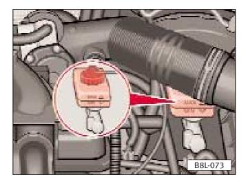
The brake fluid reservoir is on the left hand side of the engine compartment.
