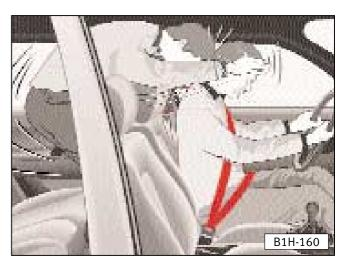
In case of a frontal collision accident, the occupants who are not belted up are thrown forwards and collide with parts of the vehicle interior, e.g. the steering wheel, instrument panel or windscreen.
