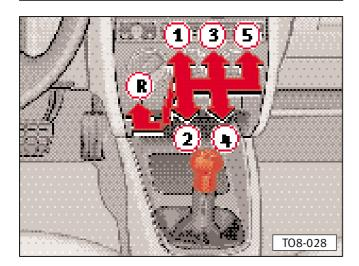
Reverse gear may only be engaged when the vehicle is stationary. When engine is running, depress clutch fully and wait a few seconds before moving gear lever, to prevent grating noises.
