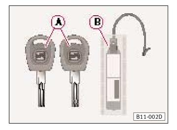
The vehicle is supplied with two keys **A** which fit all locks.
