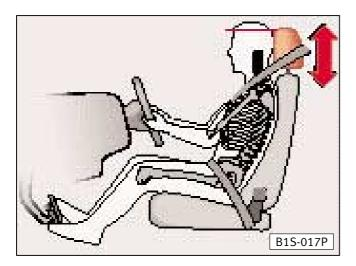
The head restraints are height adjustable and must be set to suit the size of the occupant. Correctly adjusted head restraints together with the seat belts offer effective protection. It is also possible to set the angle of the front head restraints.
