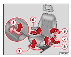
Fig. 86 Front left seat controls
