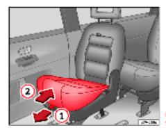
Fig. 41 Using the integrated child seat
