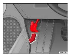
Fig. 137 Detail of footwell area on driver's side: lever for unlocking the bonnet.
