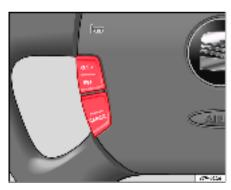
Fig. 133 Multifunction steering wheel: CCS controls
