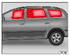
Fig. 27 Deployed curtain airbags
