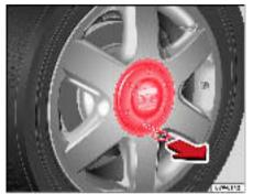
Fig. 155 Removing the hubcaps
