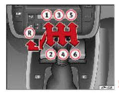
Fig. 126 Manual gearbox with shift diagram
