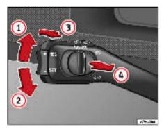
Fig. 73 Turn signal and main beam headlight
