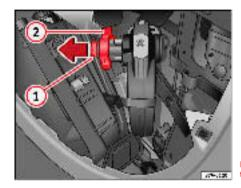
Fig. 134 Location of towing bracket
