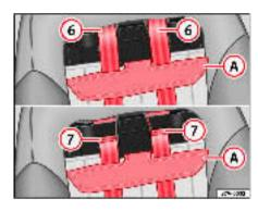
Fig. 36 Integrated child seats, adjusting the belt routing
