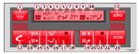
Fig. 117 Instrument panel: Climatronic controls
