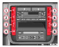
Fig. 72 Switch for hazard warning lights
