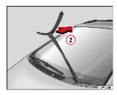
Fig. 145 Removing front wipers
