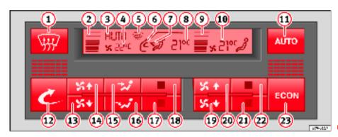
Fig. 118 Instrument panel: Climatronic controls
