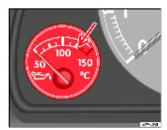
Fig. 47 Engine oil temperature gauge
