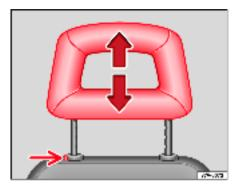
Fig. 85 Adjusting and removing the head restraints
