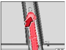
Fig. 15 Location of the belt height adjuster
