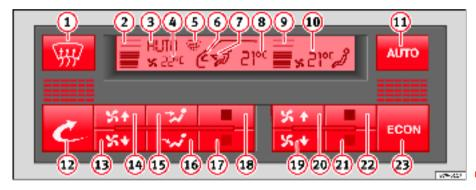
Fig. 119 Instrument panel: Climatronic controls
