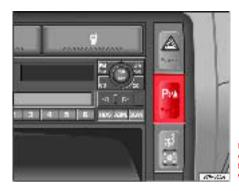
Fig. 131 Detailed view of dash panel Control button for the parking distance warning system
