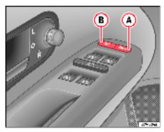
Fig. 57 Detail of driver door: central locking system button
