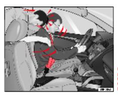
Fig. 8 The unbelted rear passenger is thrown forward violently, hitting the driver wearing a seat
