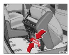
Fig. 92 Bar for removing and installing the individual seat
