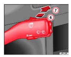
Fig. 80 Windscreen wiper and windscreen wash lever rear window wiper
