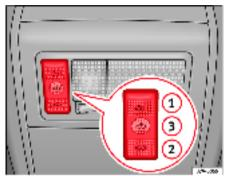
Fig. 67 Interior roof trim: control of sliding/tilting roof
