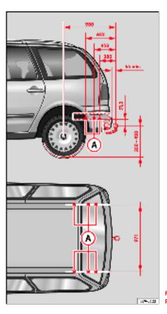
Fig. 135 Attachment points for towing bracket
