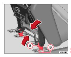
Fig. 93 Assembling seat: bar and retaining bolts
