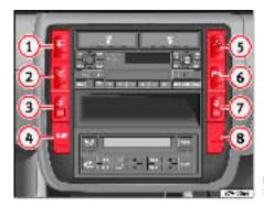
Fig. 87 Centre console: Seat heating controls
