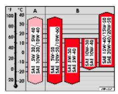
Fig. 139 Types of oil according to temperature
