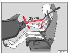
Fig. 122 Adjusting the steering wheel position
