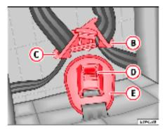
Fig. 37 Integrated child seats. closing harness belt
