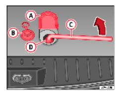
Fig. 151 Taking out the spare wheel
