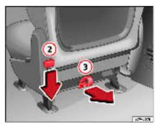
Fig. 91 Rear of seat: fold the backrest and lift seat forwards
