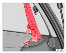
Fig. 19 Storage for the detached seat belt
