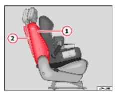
Fig. 34 Backrest adjustment when using ISOFIX child seats
