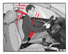
Fig. 9 Driver wearing the seat belt properly: is secured by the belt in sharp braking
