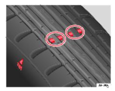
Fig. 148 Tyre tread wear
