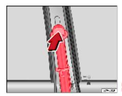
Fig. 21 Location of the belt height adjuster
