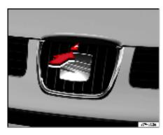
Fig. 138 Detail of radiator grille: lever for unlocking the bonnet.
