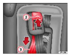
Fig. 39 Integrated child seats, adjusting harness
