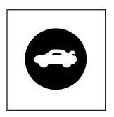
On vehicles with this feature, press the button located on the driver's door near the map pocket to open the trunk.
