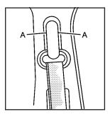
Squeeze the buttons (A) on the sides of the height adjuster and move the height adjuster to the desired position.
