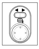
Controls for the outside power mirrors are located on the inside of the vehicle near the driver's side mirror.
