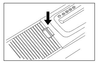
Two removable cupholders and additional storage areas are located at the rear of the shift lever. Push the button and the cover will slide back automatically for access. Slide the cover forward and lock into place to close.
