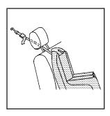
If the position you are using has an adjustable headrest or head restraint and you are using a single tether, route the tether under the headrest or head restraint and in between the headrest or head restraint posts. See *Head Restraints on page 1-8*.
