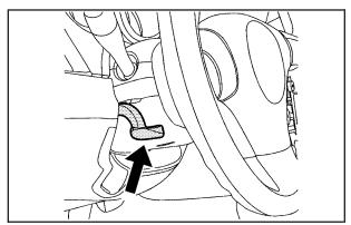
The lever is located on the left side of the steering column.
