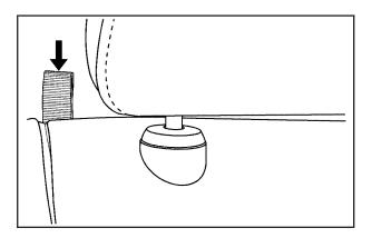
To lower the rear seatback, pull up on the seatback strap while folding the seatback down. This allows access to the trunk.
