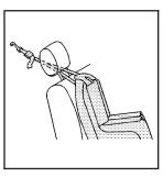
If the position you are using has an adjustable headrest or head restraint and you are using a dual tether route the tether under the headrest or head restraint and in between the headrest or head restraint posts. See *Head Restraints* on page 1-8.
