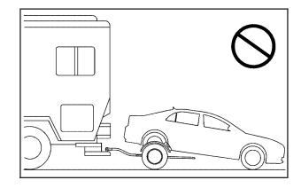
Notice: Towing the vehicle from the rear could damage it. Also, repairs would not be covered by the warranty. Never have the vehicle towed from the rear.
