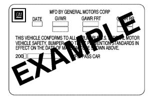
A vehicle specific Certification label is found on the rear edge of the driver's door.
