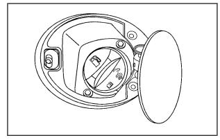
To remove the tethered fuel cap, turn it slowly counterclockwise.
