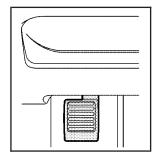
To set the parking brake, push down the parking brake pedal with your left foot. If the ignition is on, the brake system warning light will come on. See Brake System Warning Light on page 3-30.
