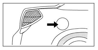
To open the fuel door, push the rearward center edge in and release and it will open.
