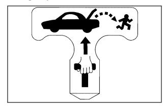
Notice: Do not use the emergency trunk release handle as a tie-down or anchor point when securing items in the trunk as it could damage the handle. The emergency trunk release handle is only intended to aid a person trapped in a latched trunk, enabling them to open the trunk from the inside.
