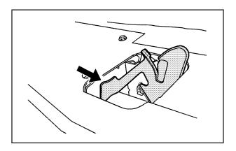
Then go to the front of the vehicle and push the secondary hood release handle toward the driver side of the vehicle.
