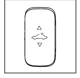
On vehicles with a sunroof, the switch is located on the headliner between the map lamps.
