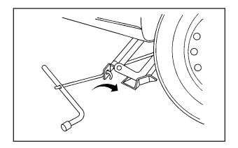
Raise the vehicle by turning the jack handle clockwise. Raise the vehicle far enough off the ground so there is enough room for the road tire to be removed.
