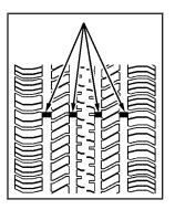
One way to tell when it is time for new tires is to check the treadwear indicators, which will appear when your tires have only 1/16 inch (1.6 mm) or less of tread remaining.
