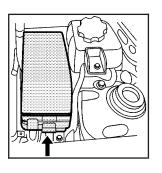
The underhood fuse block is located on the driver's side of the engine compartment, near the battery.
