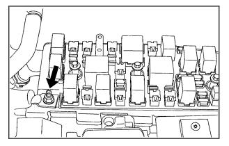
The vehicle is equipped with a remote positive (+) terminal. This is located in the engine compartment on the driver's side of the vehicle, on the underhood fuse block. See *Engine Compartment Overview on page 5-12* for more information on location.
