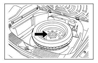
5. Place the wheel retainer bolt onto the wheel stow rod and tighten by turning it clockwise.
