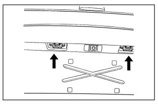
2. Turn and pull the license plate lamp forward through the fascia opening.
