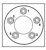
13. Tighten the wheel nuts firmly in a crisscross sequence, as shown.
