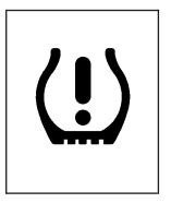
When a low tire pressure condition is detected, the TPMS illuminates the low tire pressure warning light on the instrument panel cluster.
