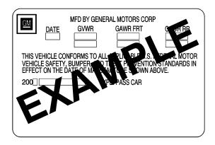
A vehicle specific Certification label is attached to the rear edge of the driver's door or the vehicle's center pillar (B-pillar) below the driver's door latch. It tells you the gross weight capacity of your vehicle, called the Gross Vehicle Weight Rating (GVWR). The GVWR includes the weight of the vehicle, all occupants, fuel and cargo. Never exceed the GVWR for your vehicle, or the Gross Axle Weight Rating (GAWR) for either the front or rear axle.
