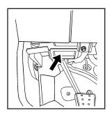
Locate the interior hood release lever. It is located below the instrument panel on the driver's side of the vehicle.
