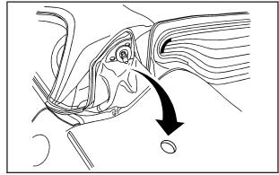
At the rear edge of the convertible top, press down on the two buttresses (C) to latch them into the top of the trunk.
