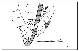
To unlatch the belt, push the button on the buckle. The belt should go back out of the way. When the safety belt is not in use, slide the latch plate up the safety belt webbing. The latch plate should rest on the stitching on the safety belt, near the guide loop.
