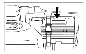
Locate the tire sealant and compressor kit on the driver side of the vehicle, near the back corner of the trunk.
