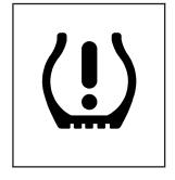
When a low tire pressure condition is detected, the TPMS turns on the low tire pressure warning light located on the instrument panel cluster.
