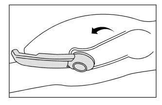
The convertible top front latch, located above the inside rearview mirror, must be unlatched. Pull the latch down and turn it counterclockwise to unlatch it.
