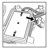
The remote positive (+) terminal is located under a red plastic cover on the engine compartment fuse block. Open the red plastic cover to access the terminal.
