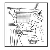
Pull down on the rear edge of the lever to release the hood latch.
