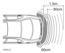
Four ultrasonic sensors, situated in the rear bumper, scan an area behind the car, searching for obstructions. If an obstruction is detected, the sensors calculate its distance from the rear of the car and communicate this information to the driver by sounding warning chimes. It is important to remember that the system is no more than an AID to parking. It is not foolproof in operation, nor is it a substitute for observation and personal judgement.
