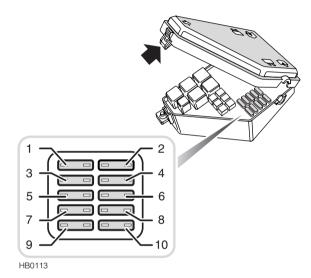
The fuse box is located to the rear of the engine compartment on the left hand side. Press the catch (arrowed in illustration) to release the cover.
