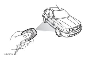
The handset has two buttons which, when pressed, send a coded radio signal to a receiver in the car. The 'padlock' symbol button activates the alarm and a plain button deactivates the alarm. On models with central door locking the 'padlock' symbol will also lock the car and the plain button will unlock the car.
