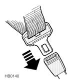
Pull the seat belt steadily over the shoulder and across the chest and, ensuring the webbing is not twisted, insert the metal tongue plate into the buckle nearest the wearer – a 'click' indicates that the belt is securely locked.
