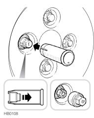
Cars with alloy wheels are fitted with one locking wheel nut on each wheel. These are visually very similar to standard wheel nuts, but can only be removed using the special tools provided.
