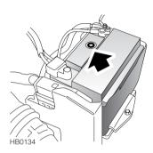
The battery is designed to be maintenance free, so topping-up is unnecessary. On the top of the battery there is a battery condition indicator (arrowed in illustration). Examine the indicator periodically to check the battery's condition. When the indicator shows:
