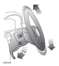
The angle of the steering column can be adjusted to suit your driving position:
