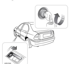
To open, use the key in the lock or, from inside the car, lift the release lever adjacent to the driver's seat. The luggage compartment light switches on automatically when the taildoor (or boot lid) is opened.
