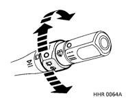
Rotate the switch clockwise to the first position to operate the rear wiper. After wiping continuously four times, the wiper continues intermittently until switched off.
