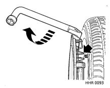
Slide the flat, wedge end of the wheel nut spanner behind the edge of the wheel trim. Working carefully around the wheel, apply a twisting action to the tool, to prise the trim from the wheel.
