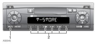
Travelstore operates on the FM waveband only and enables you to rapidly tune and store the six strongest FM radio signals in a single operation. This facility is particularly useful if you are in an unfamiliar area and have little knowledge of local transmitter frequencies.
