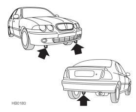
If your car is to be transported on the back of a trailer or transporter, use the recommended lashing points at the front and rear of the car only. DO NOT secure lashing hooks, 'T' bars or trailer fixings to any other part of the car.
