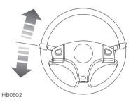
Move the lever down to indicate a LEFT turn, or up to indicate a RIGHT turn. The indicators will cancel automatically once a turn has been completed.
