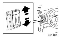
The angle of the dipped beams is affected by the distribution of passenger and luggage weight within the car. It is important that the headlights are adjusted to ensure that the point at which they meet the road surface provides adequate illumination ahead of the vehicle, without dazzling other road users.
