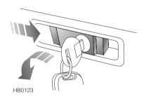
Turn the key anti-clockwise to unlock the glovebox. Squeeze the catch to the left of the lock to open (see illustration).
