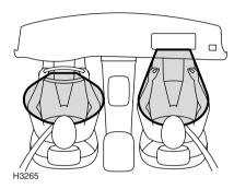
Airbag inflation is virtually instantaneous and occurs with considerable force, accompanied by a loud noise. The inflated bag, together with the seat belt restraint system, limit the movement of a front seat occupant, thereby reducing the risk of injury to the head and upper torso.
