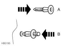
To replace the fastener, push on the pointed end (arrowed in illustration 'A') until the centre protrudes from the collar (as illustration 'B').
