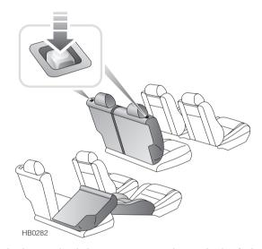
The backrest is divided into two parts; either, or both of which, can be folded forward to increase the luggage space. Press the backrest release buttons (arrowed in illustration) to release the backrest.
