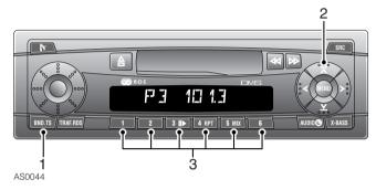
The six pre-set buttons (3) can be used to manually store up to eighteen FM stations (six each on FM1, FM2 and FMT), six MW stations and six LW stations.
