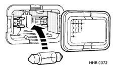
Use a small screwdriver to prise the lens from the light housing. Pull the bulb to remove.
