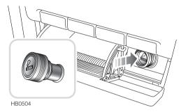
Push the top of the ashtray cover to open (see 'ASHTRAYS', page 48). With the starter switch turned to position 'I' or 'II', push the lighter in to heat up. When ready, the lighter will partially eject and can then be withdrawn for use. DO NOT hold the lighter in while it is heating – this could cause it to overheat.
