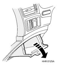
Pull down to open (for instructions showing removal and replacement of the storage container, see 'MAIN FUSE BOX', page 169).
