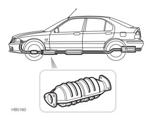
The exhaust system on your car incorporates a catalytic converter which converts poisonous exhaust emissions from the engine into environmentally less harmful gases, thereby reducing atmospheric pollution.
