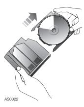
Holding the magazine as shown (arrow on magazine casing uppermost), remove each CD tray in turn.
