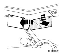
To shield your eyes from the sun, pull the visor down from the roof; the visor can be used to shield the upper part of the windscreen, or the side window as required.
