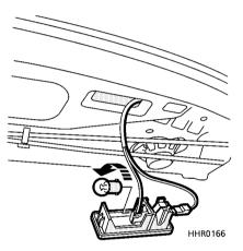
Use a small screwdriver to prise the lens from the light housing. Twist the bulb to remove.
