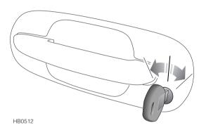
With the starter switch turned off and the driver's door locked, enter the code as follows:
