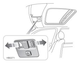
The sunroof can be operated when the starter switch is turned to position 'II' and for up to 30 seconds after the starter switch is turned off, unless a door is opened in the meantime.
