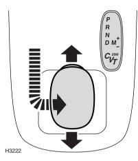
There are six predetermined gear ratios, all of which can be selected sequentially by a single forward or rearward movement of the gear selector lever, as follows:
