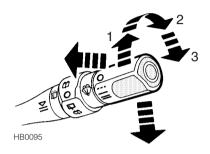
The wipers and washers will only operate when the starter switch is turned to position 'II'.
