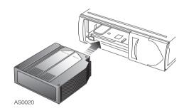
Only insert the magazine (3) in the direction of the arrow marked on the magazine casing and push it fully into the changer. Finally, close the cover.
