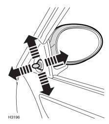
Manually operated mirrors are adjusted by moving the lever as shown in the illustration.
