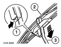
Lift the wiper arm away from the windscreen. With the blade at 90° to the arm as shown, disconnect the blade by pushing in the locking tab (1) and sliding the blade (2) down the arm (3).
