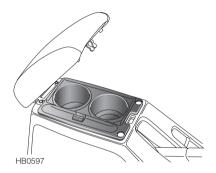
Lift the front edge of the lid to open. Stowage space is provided for a pen and two cup rests for use when the car is stationary. The cup rests can be removed from the centre armrest, to access a stowage box.
