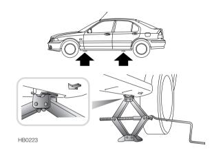
Position the jack under the jacking point nearest the wheel to be removed (note that arrows pressed into the sills identify the four jacking points). Turning the jack screw by hand, raise the jack until the jack head fits snugly around the centre of the jacking point. Ensure that the base of the jack is in full contact with the road surface.
