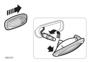
Push the lens firmly towards the front of the car to release the light unit, then withdraw the light from the wing.
