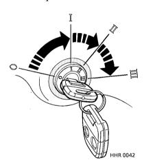
The starter switch uses the following sequence of key positions to operate the steering lock, electrical circuits and starter motor:
