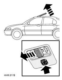
To raise the rear edge of the roof; with the sunroof closed, press the button (arrowed in illustration). To return the tilted roof to the closed position, pull the OPEN/CLOSE switch forward. 1
