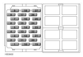
Always turn off the starter switch and the appropriate electrical circuit before removing a fuse. To remove a fuse, press the removal tweezers onto the head of the fuse and pull. Always replace a fuse with another of the same (or lower) rating. If a replacement fuse blows almost immediately, this indicates a serious electrical problem and the circuit MUST be checked by an MG Rover dealer.
