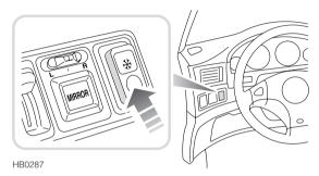
With the selector lever in 'D', press the switch on the fascia to select snow mode (the Snow mode warning light in the instrument panel will illuminate). Snow mode should be selected when moving from rest on loose or slippery surfaces. In Snow mode, the car will move off in a higher ratio, providing less torque to the road wheels, thereby reducing the possibility of wheel spin.
