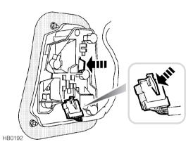
Detach the electrical connector from the back of the light unit by depressing the release catch (arrowed in inset) and then pulling the connector free.
