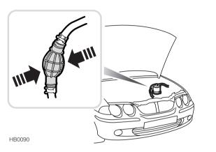
In the event of the fuel tank running dry, it will be necessary to hand-prime the fuel system (after refuelling) by squeezing the priming bulb in the engine compartment (where shown in illustration), until the bulb feels solid.
