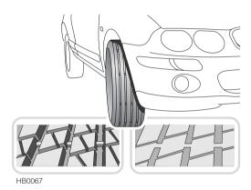
Tyres fitted as original equipment have wear indicators moulded into the tread pattern at several points around the circumference. When the tread has worn down to 1.6 mm, the indicators will come to the surface of the tread pattern, producing the effect of a continuous band of rubber across the width of the tyre.
