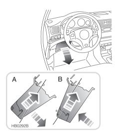
To access the interior fuse box, first remove the driver's personal storage compartment as follows (see diagram 'A'):
