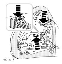
Detach the electrical connector from the back of the light unit by depressing the release catch (arrowed in inset) and then pulling the connector free.
