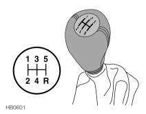
The gear positions are indicated on the gear lever knob.
