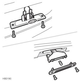
The upper part of the illustration represents the process for 4-door models, the lower part represents 5-door models.
