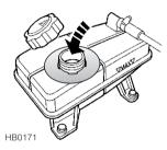
Remove the filler cap, and top-up to the MAX' mark with a 50% mixture of water and anti-freeze (see *'Coolant specification'*). Ensure the cap is tightened fully after top-up is completed.
