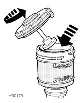
Wipe the filler cap clean before removing, to prevent dirt from entering the reservoir. Unscrew the cap 1/4 turn anti-clockwise and lift to remove. Top-up the reservoir to the 'MAX' mark using a recommended fluid.
