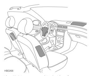
The airbag SRS incorporates a driver's airbag, front passenger airbag and optional side airbags for both front seats.
