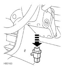
The fuel cut-off switch is a safety device which, in the event of a collision or sudden impact, automatically cuts off the fuel supply to the engine.
