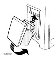
Pull out to open. To remove for emptying, open the ashtray fully and then lift the base up and outwards.
