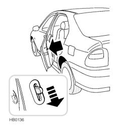
Move the locking levers on the rear doors down to engage the child locks.
