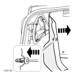
From inside the luggage compartment, remove the fastener (illustrated in inset) and pull back the moulded lining as shown.
