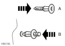
To replace the fastener, push on the pointed end (arrowed in illustration 'A') until the centre protrudes from the collar (as illustration 'B').
