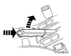
The handbrake operates on the rear wheels only. To apply the handbrake, pull the lever up. Always apply the handbrake FULLY whenever you park the car.
