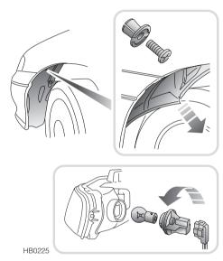
The direction indicator bulbs are accessible from behind the wheel arch liners, as follows:
