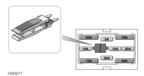
A separate module containing spare fuses of varying values is attached to one side of the main fuse box. The module contains:
