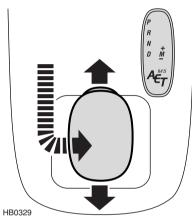
There are five predetermined gear ratios, all of which can be selected sequentially by a single forward or rearward movement of the gear selector lever, as follows:
