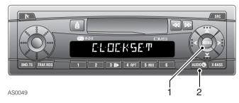
To display the time, press and hold the clock control (2). The display will be present for approximately two seconds.
