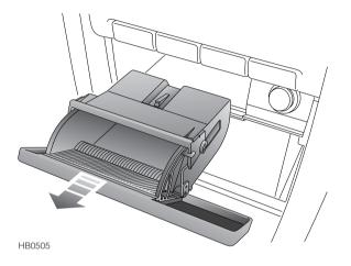
To remove for emptying, open the cover and pull out the entire ashtray unit.
