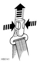
To reduce the likelihood of injury in an accident, the seat belt upper anchorage point should be adjusted so that the belt webbing crosses the shoulder, MIDWAY BETWEEN THE NECK AND THE EDGE OF THE SHOULDER.
