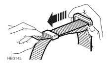
To adjust the length of the belt, turn the adjuster at right angles to the webbing (as shown in the illustration) and then pull the webbing through the adjuster to the required length.
