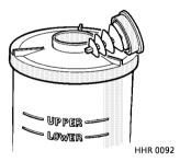
Wipe the filler cap clean to prevent dirt from entering the reservoir. Remove the filler cap and top-up to the 'UPPER' level mark with a fluid meeting Dexron IID or III specification. DO NOT OVERFILL!
