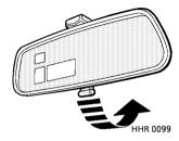
The interior mirror can be dipped to reduce glare from following vehicles. At night, move the lever at the base of the mirror forward to 'dip' the mirror. Normal visibility is restored, by pulling the lever back to its original position.
