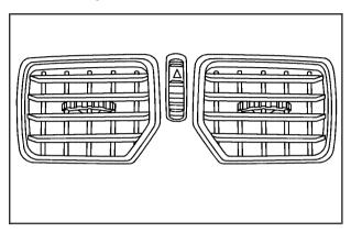
Move the thumbwheel on the vents to change the direction of the airflow. The center thumbwheel adjusts the volume of the airflow.
