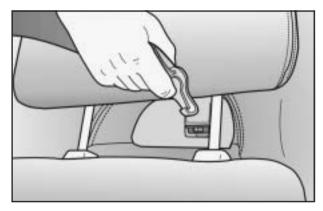
The straps from the child restraint must be threaded between the poles of the head restraint on the seat. The strap must not go around the head restraint.
