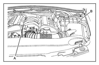
When you decide it's safe to lift the hood, you'll see the electric engine cooling fan (A) and the engine coolant reservoir (B).
