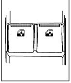
Use the switches located between the seats to operate the windows.
