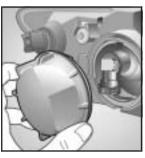
Turn the dust caps counterclockwise and remove from the rear of the headlamp assembly to gain access to the bulb.
