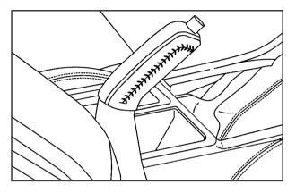
To set the parking brake, pull up on the parking brake handle without pressing the release button. If the ignition is on, the brake system warning light will come on. See *Brake System Warning Light on page 3-27*.
