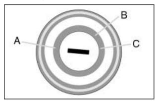
A (LOCK and ACCESSORY): This is the only position from which you can insert or remove the key. When the key is inserted and is in this position, all accessories, electrical systems, and engine are off. If the key is cycled back to this position the accessories will remain on until the key is removed. Once the key is removed the accessories will turn off. If the key is left inserted in this position, a chime will sound when the driver's
