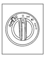
When the parking lamps are turned on, the interior instruments are automatically illuminated and you can adjust the brightness. Move the tab clockwise to increase brightness and counterclockwise to decrease brightness.
