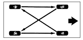
When rotating non-directional tires, always use the correct rotation pattern shown here.
