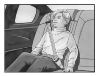
Buckle, position and release the safety belt as described in *Rear Seat Passengers on page 1-20*. Make sure that the shoulder belt crosses the shoulder.
