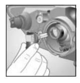
4. Remove the old bulb by twisting the bulb counterclockwise.
