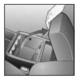
To open the armrest storage area, pull up on the latch at the front edge of the lid.
