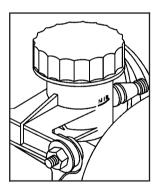
Refer to the Maintenance Schedule to determine the proper fluid. See *Owner Checks and Services on page 6-9* and *Recommended Fluids and Lubricants on page 6-13.*
