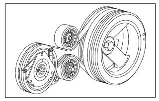
Air Conditioning Compressor Belt Routing
