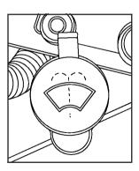
Open the cap and add washer fluid until the tank is full. Make sure the cap is secured after filling.
