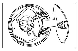
The fuel cap is located behind a hinged fuel door on the passenger's side of your vehicle.
