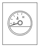
The temperature gage shows the engine coolant temperature when the ignition is on.
