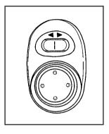
The controls for the power mirrors are located on the driver's door armrest.
