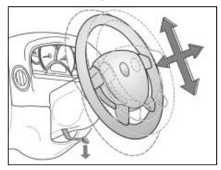
To tilt the wheel, pull the lever down. Then move the wheel to a comfortable position and release the lever to lock the wheel in place.
