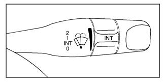
The lever on the right side of the steering column operates the windshield wipers and washer.
