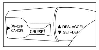
With cruise control, you can maintain a speed without keeping your foot on the accelerator. This can really help on long trips. Cruise control does not work unless the vehicle speed is at least 25 mph (40 km/h).
