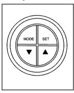
When the vehicle is stationary, hold down the MODE button while turning the ignition from LOCK to ON.
