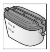
Your brake master cylinder reservoir is filled with DOT-4 brake fluid. See Engine Compartment Overview on page 5-12 for the location of the reservoir.
