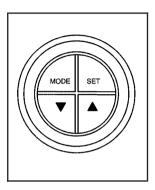
The buttons for the trip computer are located to the right of the gages and the display is located directly beneath the gages.
