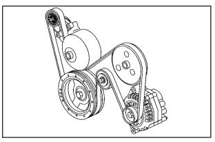
Power Steering/Generator Belt Routing
