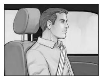
To raise the height of the head restraint, pull the head restraint up. To lower the height of the head restraint, push in the locking clip at the base of the head restraint and push the head restraint down. The locking clip needs to be pushed outboard on the driver's side head restraint and inboard on the passenger's side. The upper edge of the head restraint should be about at eye level, never at neck level. This position reduces the chance of a neck injury in a crash.
