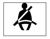
When the key is turned to ON, the safety belt light will come on and stay on for several seconds and a chime will be sounded for eight seconds, then it will flash continuously until the driver's belt is buckled.
