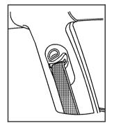
To move it up or down, squeeze the adjuster as shown and move it to the desired position. After you move the adjuster to where you want it, try to move it without squeezing it, to make sure it has locked into position.
