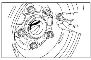
Put the wheel nuts back on with the rounded end of the nuts toward the wheel. Tighten each nut by hand until the wheel is held against the hub.
