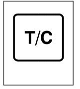
To turn the system off, press the T/C button. On manual transmission vehicles the button is located on the driver's side of the center console. On automatic transmission vehicles the button is located on the passenger's side of the shift lever.
