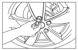
Remove each wheel nut cap individually with the wheel nut cap tool provided. Insert the nut cap tool into the nut cavity, squeeze the tool to grasp the nut cap, and pull out to remove it. Store the nut caps in a clean area to avoid dirt getting into them.
