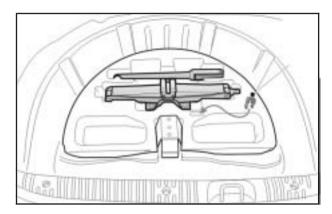
Remove the jack, wheel wrench, and nut cap removal tool from storage. Your vehicle's jack, wheel wrench, and nut cap removal tool are stored in a container in the floor, under the spare tire.
