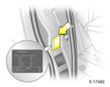
The Gross Vehicle Weight and Gross Train Weight can be found on the vehicle identification plate, which is located on the right-hand door pillar.
