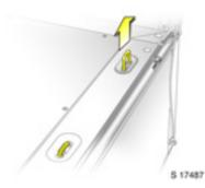
Pull up the lashing eyes as required. Secure heavy objects with lashing straps attached to the lashing points. If heavy loads slip when the vehicle is braked heavily or driven around a bend, the handling of the vehicle may change.
