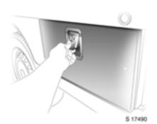
To open, pull latch and lower flap. Upon closing, ensure the flap is pushed firmly until an audible click is heard.
