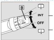
Turn the knob **B** to operate the rear window wiper.
