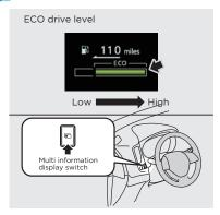
This function displays how fuelefficiently you are driving under different driving conditions. To show, press the multi information display switch.
