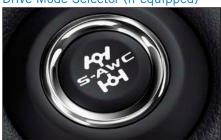
The drive mode can be switched by pressing the drive mode button while the ignition switch is in the ON position.
