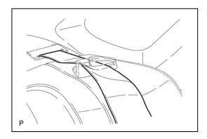
(2) Disconnect the rear seat outer belt assembly RH from the rear seat shoulder belt guide RH.
