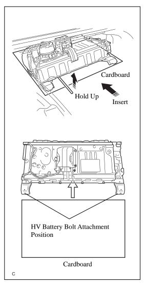
(7) Pull the cardboard and HV battery together to the middle of the luggage compartment.
