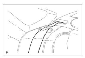
(3) Disconnect the rear seat inner with center belt assembly LH from the rear seat shoulder belt guide LH.
