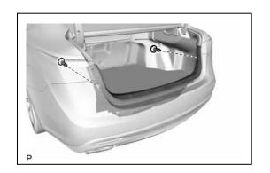
(2) Disengage the 4 clips and 3 guides to remove the rear floor finish plate as sown in the illustration.
