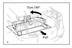
(15) Using a suitable adaptor such as a rope, remove the HV battery while tilting the HV battery.
