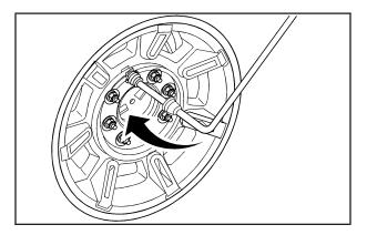
5. Try to move the tire back and forth slightly to make sure it is secure.
