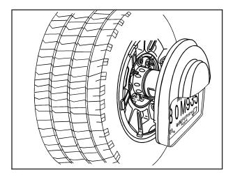
Slide the license plate holder onto the spare or flat tire. Secure it from the back of the tire carrier with the wing nut.
