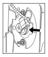
Locate the lamp assembly behind the front bumper through the wheel opening.
