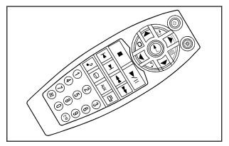
$\stackrel{(}{\cup}$  (Power): Press this button to turn the video screen on and off.
