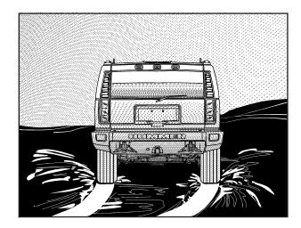
What is the worst time for this? Wet ice. Very cold snow or ice can be slick and hard to drive on. But wet ice can be even more trouble because it can offer the least traction of all. You can get wet ice when it is about freezing,  $32^{\circ}F$  (0°C), and freezing rain begins to fall. Try to avoid driving on wet ice until salt and sand crews can get there.
