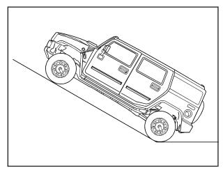
Design specifications required a minimum gradeability of 60% (31°) slope, with the vehicle fully loaded, on high friction surfaces at 6 mph (9.7 km/h). The vehicle is expected to traverse this grade only for short durations. Never stop and idle the vehicle or park it on this grade.
