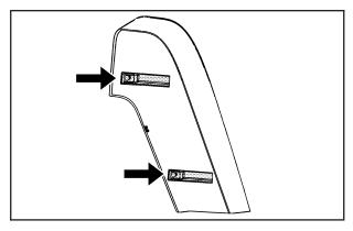
1. To access the jack pull on the two latches to remove the trim cover.
