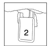
3. To unlatch the rear of the seat from the floor, pull up on the release lever labeled 2, at the rear of the seat, and lift the rear of the seat up from the floor.
