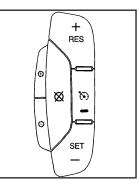
The cruise control buttons are located on the left side of the steering wheel.
