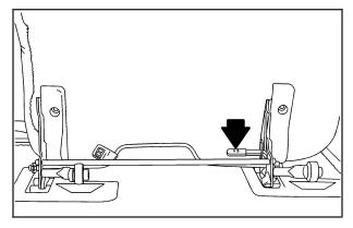
4. Push down on the seat firmly. Try pulling it up to be sure it is locked into place.
