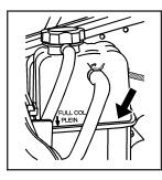
The coolant surge tank is located in the engine compartment on the passenger's side of the vehicle. See *Engine Compartment Overview on page 5-12* for more information on location.
