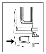
1. Locate the affected taillamp which is behind and under the bumper.
