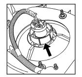
Turn the bulb/ socket retainer counterclockwise to unlock the bulb/socket.
