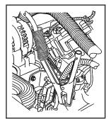
The remote positive (+) terminal is located near the engine accessory drive bracket. On some vehicles, the terminal may be covered by a red plastic cover. To access the remote positive (+) terminal, open the cover, if equipped.
