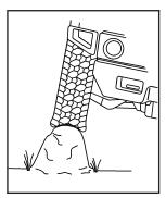
Do not straddle large rocks; drive over them, letting the tire cover the rock. The tread of the tire is thicker and tougher than the sidewall of the tire and is more resilient to impact than underbody components.
