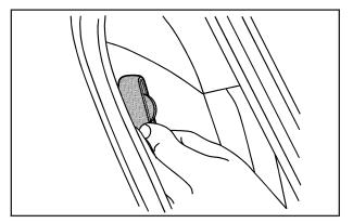
1. Remove the guide from its storage pocket on the side of the seat.
