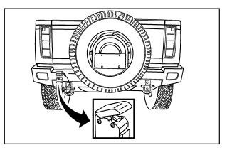
Lift up on the latch on the left side of the vehicle to release the spare tire carrier from the vehicle. The handle will stay in the raised position until the spare tire carrier is closed and latched properly.
