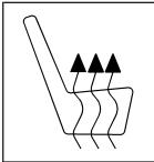
Driver's Side RSA Heated Seat Button shown On vehicles with rear outboard heated seats, the buttons used to control this feature are located on the Rear Seat Audio (RSA) panel. (Heated Seat): To heat the seat cushion, press the button with the heated seat symbol.
