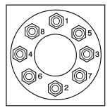
15. Tighten the nuts firmly in a crisscross sequence as shown by turning the wheel wrench with the wheel wrench extender clockwise.
