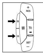
Your vehicle has a Driver Shift Control (DSC). The DSC controls the vehicle's transmission and vehicle speed while driving down hill or towing a trailer by allowing you to select a desired range of gears.
