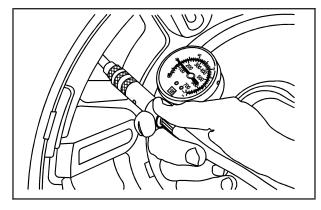
The accessory inflator hose also has a built-in air pressure gage. As soon as you start to inflate an object it will automatically read the current pressure.
