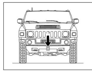
Your vehicle is equipped with a front mounted receiver.
