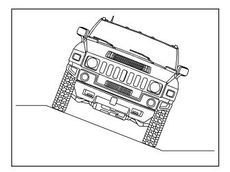
Also, your vehicle should be able to traverse a 40% (22°) side slope at 6 mph (9.7 km/h) while fully loaded on high friction surfaces.
