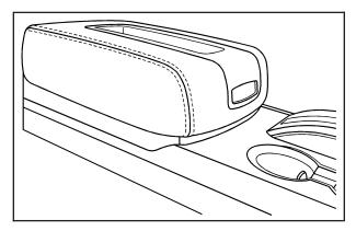
Your vehicle has a center console located between the front seats. To open, press the button and lift up.
