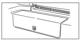
To access the jack, remove the cover, unlock it and then pull the cover off.
