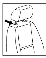
Pull the head restraint up to raise it. To lower the head restraint, press the release button, located on the top of the seatback, while you push the head restraint down.
