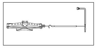
**Front Flat Tire:** Attach the jack handle with the hook end connected to the hole on the jack. Slide the wheel wrench onto the jack handle extension.
