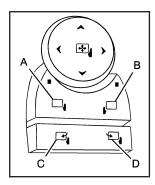
If your vehicle has outside power foldaway mirrors, the controls are located on the driver's door armrest.
