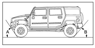
The HUMMER H2 has an approximate approach angle (A) of  $42^{\circ}$  and a departure angle (B) of  $37^{\circ}$ .
