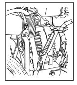
The remote negative (–) terminal is located on the engine accessory drive bracket and is marked GND (Ground).
