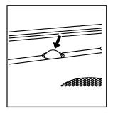
The solar sensor, located in the defrost grille in the middle of the instrument panel, monitors the solar radiation. Do not cover the solar sensor or the system will not work properly. There is also an exterior temperature sensor located behind the front grille. This sensor reads the outside air temperature and helps maintain the temperature inside the vehicle. Any cover on the front of the vehicle could cause a false reading in the displayed temperature.
