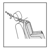
If the position you are using has an adjustable headrest or head restraint and you are using a dual tether, raise the headrest or head restraint and route the tether under the headrest or head restraint and in between the headrest or head restraint posts.
