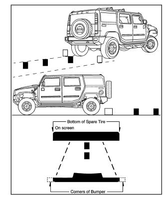
*Notice:* The spare tire extends farther away from rear of the vehicle than the trailer hitch shown on rear vision camera display. Your spare tire could hit an object even though there appears to be enough distance on the display between the trailer hitch and objects behind you causing vehicle or property damage. Do not use this system to judge the distance between the spare tire and objects behind you.
