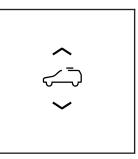
The vehicle may have a power sliding sunroof. The ignition must be on or in the accessory position, or Retained Accessory Power (RAP) must be active.
