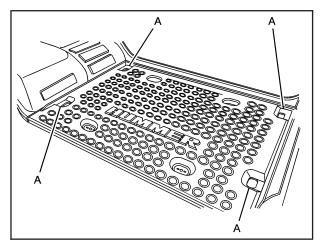
Your vehicle also has four cargo-area floor drains (A) located under the cargo mat, if it has this feature, near the sides of the cargo area. These drains should be cleaned periodically to allow water to exit the cargo area.
