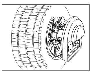
6. Slide the license plate holder onto the spare or flat tire. Secure it from the back of the tire carrier with the wing nut.
