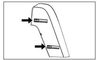
7. Replace the trim cover. Make sure the latches are pushed down.
