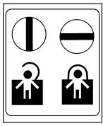
The rear door security locks are located on the inside edge of each rear door. You must open the rear doors to access them. The label depicting lock and unlock positions is located near the lock.
