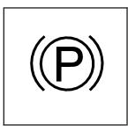
A chime will activate and the warning light will flash when the parking brake is applied and the vehicle is moving at least 3 mph (5 km/h) for at least three seconds.
