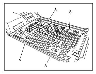
There are four oval shaped openings (A) in the cargo bed that allow access to four tie downs. You can use these tie downs to secure cargo.
