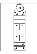
A power window switch is located on the armrest of each side door. The switches operate while the ignition is in ON/RUN or ACC/ACCESSORY or while Retained Accessory Power (RAP) is active. See Retained Accessory Power (RAP) on page 2-29.
