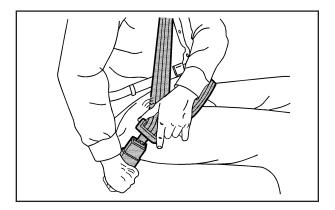
3. Push the latch plate into the buckle until it clicks. Pull up on the latch plate to make sure it is secure. If the belt is not long enough, see *Safety Belt Extender on page 1-35*.
