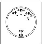
The transfer case dial is located to the right of the instrument panel cluster. Use this switch to shift into and out of the different Full-Time Four-Wheel Drive modes.
