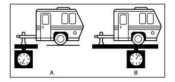
The trailer tongue weight (A) should be 10 percent to 15 percent of the total loaded trailer weight (B), up to a maximum of 600 lbs (272 kg) with a weight carrying hitch. The trailer tongue weight (A) should be 10 percent to 15 percent of the total loaded trailer weight (B), up to a maximum of 1,000 lbs (454 kg) with a weight distributing hitch.
