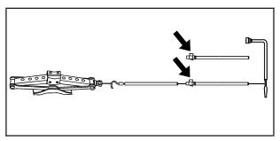
**Rear Flat Tire:** Assemble the jack together with the jack handle and the jack handle extensions.
