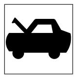
2. Pull the handle with this symbol on it. It is located inside the vehicle to the lower left of the steering column.
