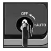
To turn off the right front passenger's frontal air bag, insert your ignition key into the switch, push in, and move the switch to the off position.
