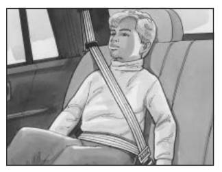
Buckle, position and release the safety belt as described in Rear Seat Passengers on page 1-26. Make sure that the shoulder belt crosses the shoulder.
