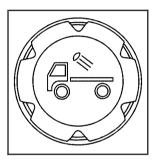
Press this button to turn the cargo lamps on and off.
