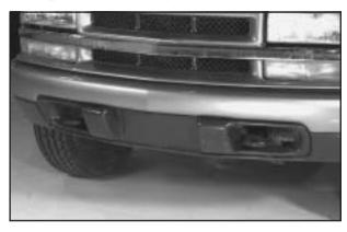
Your vehicle may be equipped with recovery hooks. The hooks are provided at the front of your vehicle. You may need to use them if you are stuck off-road and need to be pulled to some place where you can continue driving.
