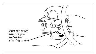
The lever to tilt the steering wheel
