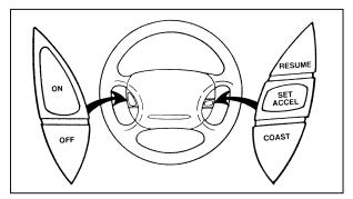
The cruise control buttons on the steering wheel
