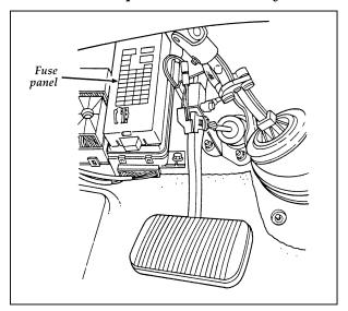
The instrument panel fuse panel location
