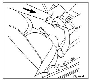
Setting the retractor to automatic locking mode
