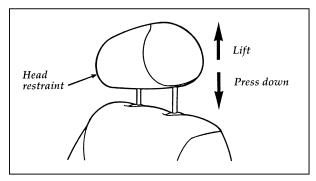
Adjusting the standard head restraint
