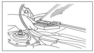
Installing the new filter
