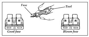
Fuse puller tool and fuse
