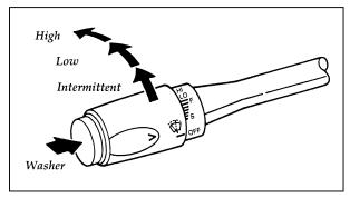
The variable interval wiper on the turn signal lever
