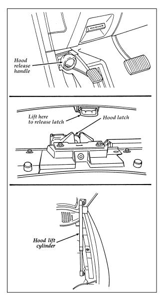
The hood release, hood latch, and lift cylinder assembly
