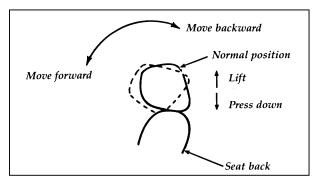
Adjusting the four-way head restraint
