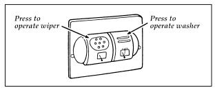
The liftgate window wiper and washer switches
