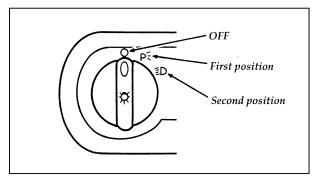
The knob for the headlamps, parking lamps, license plate lamps and tail lamps
