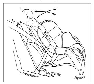
Checking that the seat is secure
