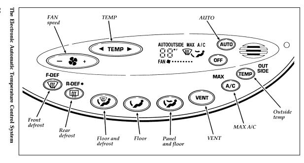
To turn your EATC on, press the AUTO button or any of the six manual override buttons along the bottom of the control.
