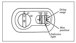
The autolamp system on the left side of the instrument panel
