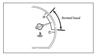
Engine coolant temperature gauge
