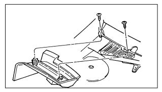
Removing the water shield
