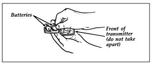
Replacing the batteries
