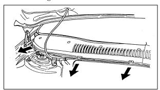
Removing the vacuum hose clips
