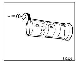
The autolight system can turn on the headlights automatically when it is dark, turn off the headlights when it is light, and keep the headlights on for up to 45 seconds after you turn the key to OFF and open any door then close all the doors.
