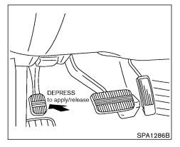
**To apply:** Fully depress the parking brake pedal.
