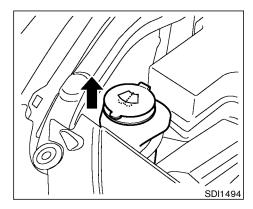
Add fluid when the low washer fluid warning light comes on. Add a washer solvent to the water for better cleaning. In the winter season, add a windshield washer anti-freeze. Follow the manufacturer's instructions for the mixture ratio.
