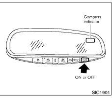
When the COMPASS switch is in the ON position, the compass display will indicate the direction the vehicle is heading.
