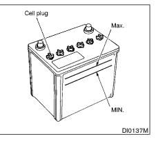
Check the fluid level in each cell. It should be between the MAX and MIN lines.
