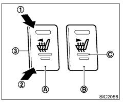
The front seats are warmed by built-in heaters. The switches located on the center console can be operated independently (driver side seat (A) and front passenger side seat (B)) of each other.
