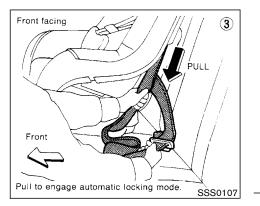
Pull on the shoulder belt until all of the belt is fully extended. At this time, the belt retractor is in the automatic locking mode (child restraint mode). It reverts back to emergency locking mode when the belt is fully retracted.
