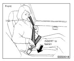
THREE-POINT TYPE SEAT BELT WITH RETRACTOR
