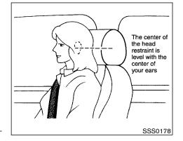
Adjust the head restraints so the center is level with the center of your ears.
