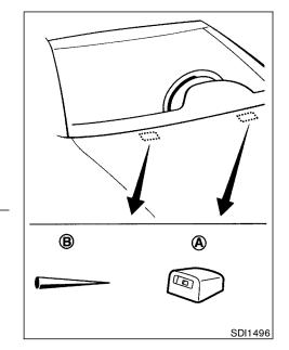
If you wax the surface of the hood, be careful not to let wax get into the washer nozzle. This may clog the nozzle (A) that could cause improper windshield washer operation. If wax gets into the nozzle, unclog it with a needle or small pin (B).
