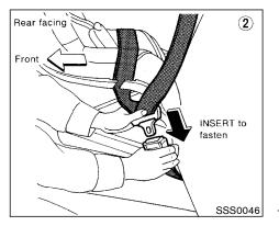
Route the seat belt tongue through the child restraint and insert it into the buckle until you hear and feel the latch engage.
