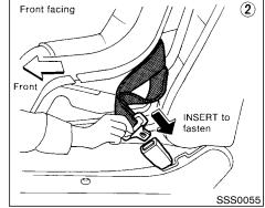
2. Route the seat belt tongue through the child restraint and insert it into the buckle until you hear and feel the latch engage. Be sure to follow the child restraint manufacturer's instructions for belt routing.
