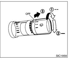
The rear window wiper and washer operate when the ignition switch is in the ON position.
