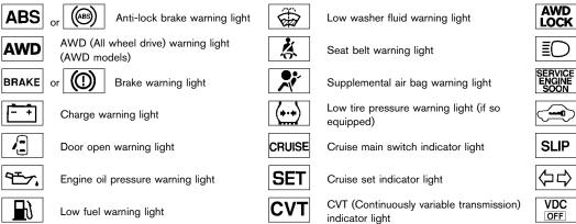
Apply the parking brake and turn the ignition key to ON without starting the engine. The following lights will come on:
