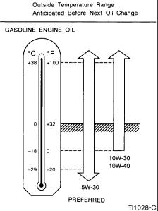
SAE 5W-30 viscosity oil is preferred for all ambient temperatures. SAE 10W-30, 10W-40 viscosity oil may be used if the ambient temperature is above  $0^{\circ}F(-18^{\circ}C)$ .
