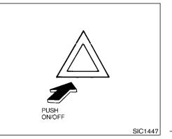
Push the switch (located on the right side of the meter panel) on to warn other drivers when you must stop or park under emergency conditions. All turn signal lights will flash.
