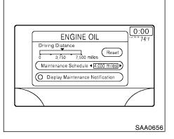
To set the maintenance interval, select the "Maintenance Schedule" key by using the joystick and push the joystick to right or left.
