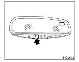
Using both hands, simultaneously press and hold both the HomeLink<sup>®</sup> button you want to program and the hand-held transmitter button.
