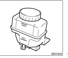
Check the fluid level in the reservoir. If the fluid is below the MIN line or the brake warning light comes on, add **DOT 3** fluid up to the MAX line. If fluid must be added frequently, the system should be thoroughly checked by your NISSAN dealer.
