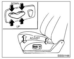
Seat lifter (if so equipped for driver's seat)
