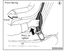
4. Allow the belt to retract. Pull up on the belt to remove any slack in the belt.
