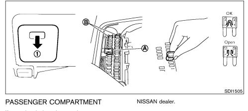
If any electrical equipment does not operate, check for an open fuse.
