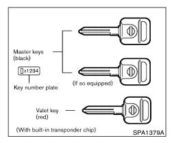
You can only drive your vehicle using the master or valet keys which are registered to the Nissan Vehicle Immobilizer System components in your vehicle. These keys have a transponder chip in the key head.
