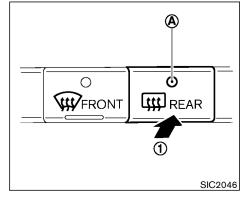
To defog/defrost the rear window glass and outside mirrors (if so equipped), start the engine and push the switch on (1). The indicator light (a) will come on. Push the switch again to turn the defroster off.
