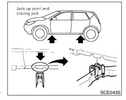
Jacking up vehicle and removing the damaged tire
