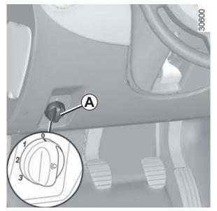
Control **A** is used to adjust the height of the headlight beams according to the load.
