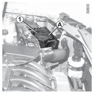
Battery 1 does not require any maintenance.
