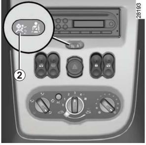
To deactivate the passenger airbag, with the ignition off, press and turn button 1 to the OFF position.
