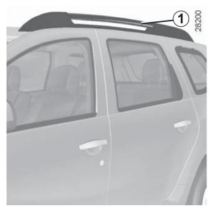
When these are fitted to the vehicle, you can transport luggage or additional accessories (bike rack, ski rack, etc.) on a roof rack or on transverse roof bars attached to the longitudinal roof bars 1 or directly on these bars.
