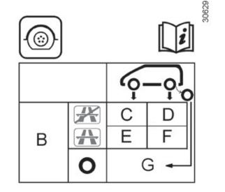
**F**: tyre pressures for the rear wheels (motorway).
