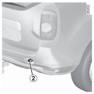
These towing points may only be used for towing: never use them for lifting the vehicle directly or indirectly.
