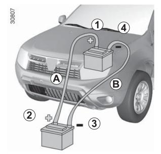
Connect the positive (+) lead **A** to (+) terminal **1** of the discharged battery, then to (+) terminal **2** of the battery supplying the current.
