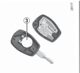
Replace battery 3 according to the direction marked on the cover.
