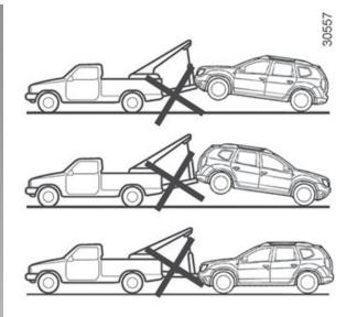
You must never tow a 4-wheel drive vehicle, irrespective of the mode selected, if one of the 4 wheels is in contact with the ground (except for off-road recovery). Risk of mechanical damage.
