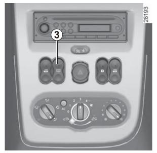
Heated rear screen With the engine running,
