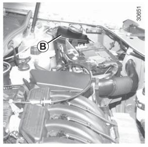
Fuses in engine compartment *B*Some functions are protected by fuses located in the engine compartment (unit *B*).
