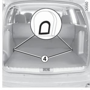
Attach the hook on the belt to one of the rings 3 (4x2 version) or 4 (4x4 version).
