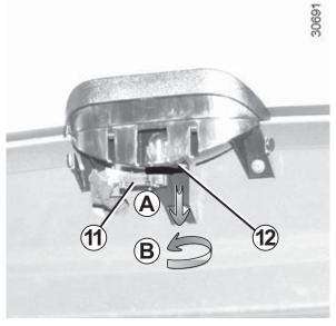
Unclip tab **12** carefully (movement **A**) and turn it an eighth of a turn (movement **B**) to release the bulb holder **11**.
