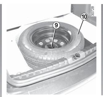
**Note**: ensure that the emergency spare wheel or punctured wheel and the wheel tray are correctly positioned so that the luggage compartment carpet can be properly fitted.
