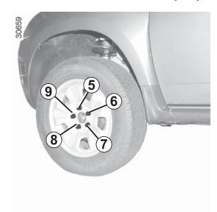
Tighten the bolts, checking that the wheel is correctly positioned on its hub and lower the jack.
