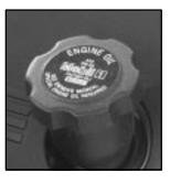
The engine oil fill cap is on top of the passenger's side valve cover.
