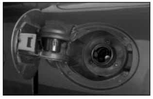
While refueling, place the cap in the holder on the fuel filler door to prevent damage to your vehicle's finish.
