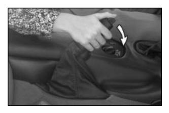
To release the parking brake, hold the brake pedal down. Hold the release button in as you move the parking brake lever all the way down.
