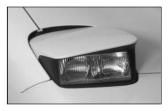
The headlamp doors are designed to open when you turn the headlamps on, and close when you turn the headlamps and parking lamps off. If you turn the headlamps on, then turn the headlamp switch back to the parking lamps setting, the headlamp doors will stay open.
