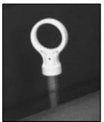
The engine oil dipstick is next to the coolant surge tank. The dipstick handle is a round, yellow loop. Turn off the engine and give the oil a few minutes to drain back into the oil pan. If you don't, the oil dipstick might not show the actual level.
