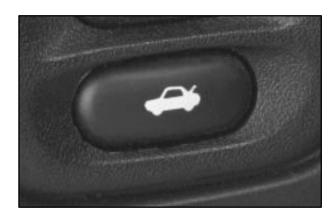
To use the remote hatch/trunk lid release on automatic transmission vehicles, your vehicle must be in PARK (P) or NEUTRAL (N). For manual transmissions, set the parking brake. See "Parking Brake" in the Index.
