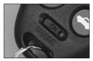
You can turn on the passive feature by moving the transmitter's slider switch to ON. Now, when you move toward your vehicle with the key fob transmitter, the system will automatically disarm your theft-deterrent system and unlock the driver's door or both depending on how the system is programmed. If it's dark enough outside, your interior lamps will come on.
