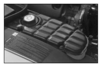
The coolant surge tank is in the engine compartment behind the passenger's side headlamp.
