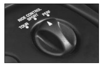
This switch is on the center console. Turn it to select the suspension characteristic of your choice.
