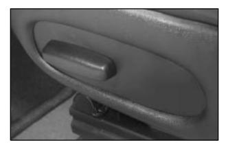
The switch for the power seats is located on the side of each seat, near the base.
