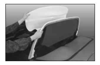
3. Lift upward on the front edge (A) of the convertible top off of the windshield frame. Then lift upward on the rear edge (B) of the convertible top to be vertical off the storage compartment lid (C). The front edge (A) and rear edge (B) should be straight up and down.
