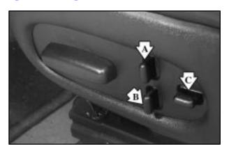
In addition to the power seat control, there are three other switches that help you change the shape of the seat. There are two lumbar supports for the middle (A) and lower (B) back. There's also a side bolster switch (C) that adjusts the sides of the seat around you to give you more lateral support.
