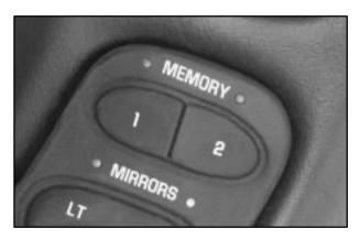
MEMORY can store and recall the settings for the driver's seat position, the outside rearview mirror positions, comfort control temperature, fan speed and mode settings, telescopic steering wheel (if equipped), radio presets, tone, volume, playback mode (AM/FM, tape or CD), last displayed station, compact disc position and tape direction.
