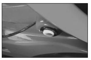
4. Tilt the driver's seatback forward and press the storage compartment release button located on the underside of the storage compartment lid (C) behind the driver's seat. Then raise the storage compartment lid (C). While attempting to raise the lid, if the lid does not release and you hear three chimes, check to make sure the trunk lid is closed. Also, the lid will not release if the alarm is turned on or the trunk lid is open.
