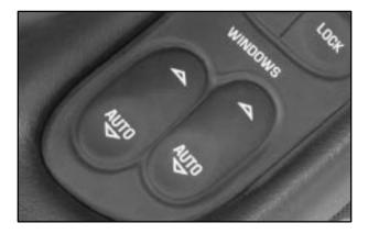
Both the driver's and passenger's window switches will have the express-down feature. Tap AUTO and immediately release. The window will lower completely. To stop the express-down feature from lowering the window completely, simply tap the switch again.
