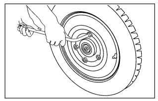
2. Use the wheel wrench to loosen all the wheel nuts. Do not remove them yet.
