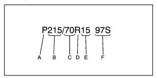
(A) Passenger (P-Metric) Tire: The United States version of a metric tire sizing system. The letter "P" as the first character in the tire size means a passenger vehicle tire engineered to standards set by the U. S. Tire and Rim Association.
