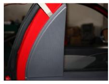
3.2. Pry out the protective cover of door inner armrest groove with slotted screwdriver, expose the fixing screw.
