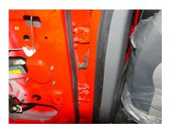
3.13. Remove the fixing bolts of rear door and hinge with 10# socket wrench, remove the rear door assembly.
