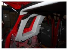
4.7. Remove the rear seat belt upper and lower fixing point and rear seat fixing clip with 17# socket wrench.
