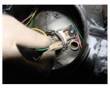
3.9. Screw off the turn signal lamp holder by hand and can replace the turn signal lamp bulb.
