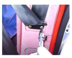
3.9. Remove the seat belt upper fixing point bolt with 17# socket wrench.
