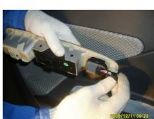
3.10. Pry out the door inner panel from edge with the plastic screwdriver.
