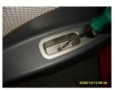
3.4. Pry out the window regulator switch with slotted screwdriver, pull off the connector of window regulator and remove it.
