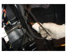
1.6. Remove the fixing bolt of anti-theft controller with 10# socket wrench, and then remove its connector.
