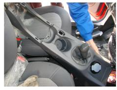
1.2. Remove the three fixing screws of instrument panel with cross screwdriver, remove the top cover of instrument panel.
