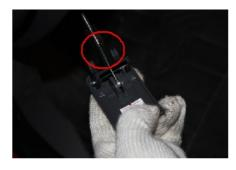
6.1.2. Pull out of the engine hood cable handle and remove the engine hood cable from the slot of pull rod.
