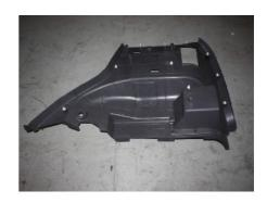
4.5. Pry out the pillar C upper panel with plastic screwdriver.
