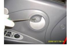
3.5. Remove the five fixing screws of door inner panel with cross screwdriver (two screws on panel front surface and three screws on panel side surface).
