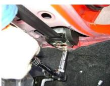
3.8. Remove the seat belt guide plate with cross screwdriver.
