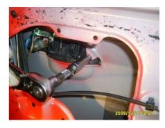
3.19. Remove the three screws fixing the lock cylinder with cross screwdriver, remove the lock cylinder.
