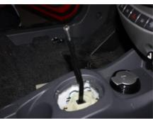
2.5. Lift up the rear part of center console and pull the rear part to remove the center console.
