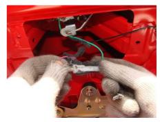
3.1.3. Remove the screws on the upper lock with cross ratchet wrench.
