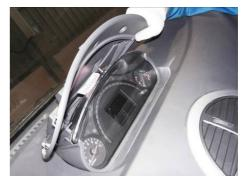
1.5. Remove the two fixing screws connecting the dashboard and instrument panel body with cross screwdriver.
