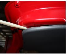
2.2. Remove the fixing bolts of license plate lamp trim board with 10# socket wrench; remove the license plate lamp trim board.
