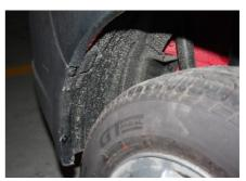
3.4. Apply the force vertical to fender surface to outwards to separate the bumper and fender clips and remove the bumper.
