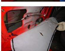
3.10. Remove the door outside handle fixing nuts with 10# socket wrench, remove the door outside handle.
