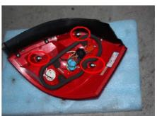
6.3. Pull off the tail lamp wiring harness connector and remove the tail lamp assembly.
