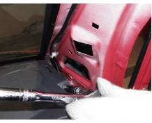
1.22. Remove the instrument panel body.
