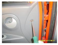
3.6. Pry out the door inner panel from edge with the plastic screwdriver.
