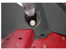
4.3. Remove the back doorsill pressure plate with cross screwdriver.
