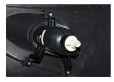
5.3. Rotate the rear fog lamp holder in anticlockwise direction to remove the rear fog lamp bulb.
