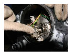
3.8 Pull off the front position lamp wirning harness connector and remove the front position lamp bulb.
