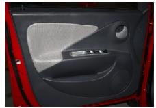
3.9. Pull out the exterior rear view mirror adjusting switch (only driver side) and window regulator control switch connector.
