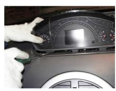
1.7. Pull off the harness connector on instrument panel body and remove it.
