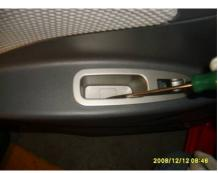
3.3. Remove the fixing screw of the door inner armrest with cross screwdriver.o
