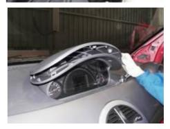
1.3. Loosen the five screws on lower cover of instrument panel with cross screwdriver.
