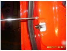
3.20. Remove the two screws that fix the lock cylinder with cross screwdriver, remove the lock cylinder.
