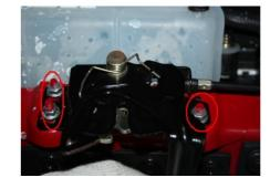
5.1.2. Remove the engine hood lock cable return spring from the engine hood lock assembly and remove the cable.
