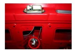
3.1.2. Disconnect the connector on upper lock body.
