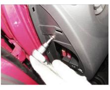
1.21. Remove the fixing bolt between body sheet metal and the instrument panel body beside speaker with 10# socket wrench.
