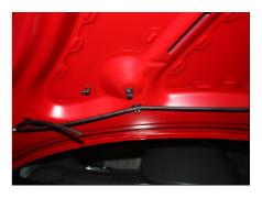
3.1.2. Press down the water nozzle clip under the engine hood, and then push it up while removing the noozle outward.
