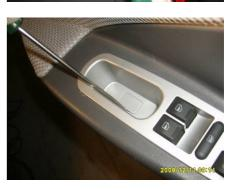
3.7. Remove the screw that fix the door inner armrest with cross screwdriver.
