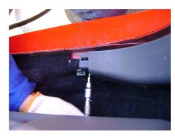
1.2. Use a plastic screwdriver to pry out the Bpillar upper panel.
