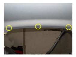
1.6. Remove the four doors and back door weather strips.
