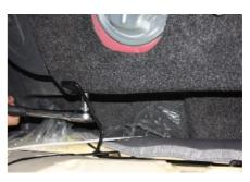
3.2. Remove the cushion after the removal of four fixing bolts.
