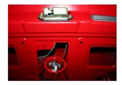
4.1.2. Push the lock cylinder out and remove it.
