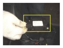
7.1.2. Remove the fixing screws of control motor and remove the motor.
