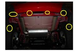
3.3. Use a 7# socket wrench to loosen the screws connecting the fender and the bumper.
