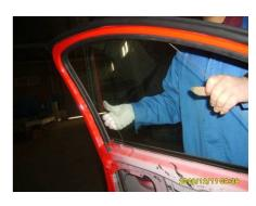
3.16. Remove the five screws that fix the window regulator with 10# socket wrench.
