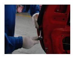
3.11. Connect the battery and lower the window glass at a proper position (let the glass fixing screws be exposed on the two installation holes as shown in figure) and remove the two screws that fix the glass with cross screwdriver, remove the glass carefully.
