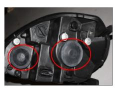
3.4. Disconnect the connector of high and low beam lamp holder.
