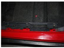
3.3. Remove the fixing bolts of rear doorsill with cross screwdriver and remove the rear doorsill pressure plate.
