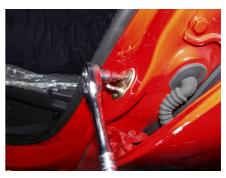
3.21. Use 13# socket wrench to remove the four fixing screws of the hinge that fix the vehicle door, remove the door.
