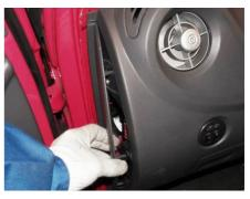
1.20. Remove the fixing screws on two sides of instrument panel body with cross screwdriver.
