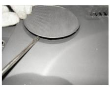
1.16. Remove the speaker body with slotted screwdriver.
