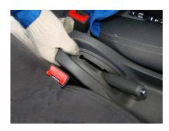
2.2. Use cross screwdriver to remove the front fixing screws of the central console assembly.
