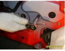
3.17. Pull off the window regulator connector and take out the window glass regulator assembly.
