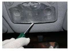
1.2. Remove the three fixing screws of the front ceiling lamp.
