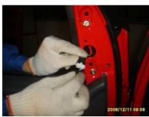
3.3. Remove the three fixing nut of exterior rear view mirror with 10# socket wrench, remove the exterior rear view mirror.
