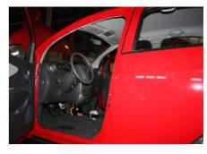
3.2. Pry out the front doorsill pressure plate with plastic screwdriver.
