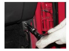
1.19. Remove the panel on two sides of instrument panel body.
