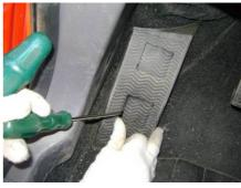
2.5. Remove the footrest with 10# socket wrench.
