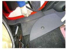
4.2. Remove the seat belt bolt with 17# socket wrench.
