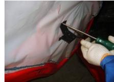
3.9. Remove the anti-water protective layer.
