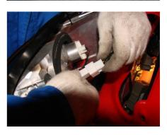
6.4. Rotate the bulb seat anti-clockwise by hand to remove the bulb.
