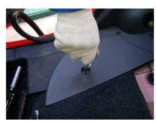
3.4. Remove the seat belt lower fixing bolt with 17# socket wrench.
