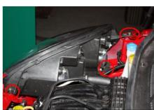
3.3. Open the headlamp high beam holder shield by hand.
