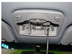
1.3. Disconnect the harness connector and remove the front ceiling lamp assembly.
