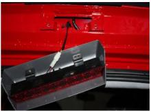
5.1.2. Remove the cover and disconnect the connector; remove the high mount brake lamp.
