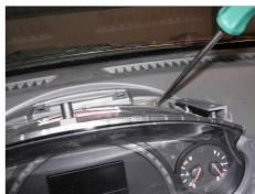
1.6. Pry out the dashboard body with slotted screwdriver.
