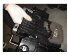
8.1.4. Remove the evaporator core.
