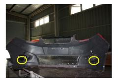
3.7. Use plastic screwdriver to pry out the edges of lower air intake grille to remove it.
