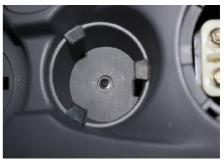
2.4. Use plastic screwdriver to pry open the gearshift handle cover and rotate the gearshift handle in anti-clockwise direction to remove it.
