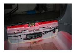
4.4. Remove the lower panel fixing bolt with cross screwdriver and remove the lower panel.
