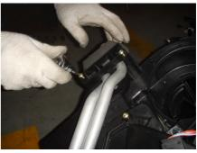
4.1.5. Tear off the sponge around the water inlet and outlet pipe and remove the heater exchanger.
