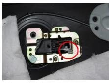
3.12. Remove the two screws of front door armrest fixing bracket with cross screwdriver.
