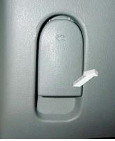
2. Push upward of the claw to lift the engine coping.
