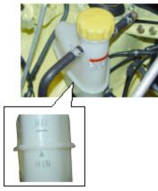
When engine is cold, coolant shall be within MAX and MIN scale on expansion tank. Level rises with engine temperature increasing and falls with engine cooling. If coolant level is under MIN scale, add anti-freezing mixture of 50% water and 50% glycol to improve anti-freezing and antisepsis performance.
