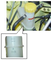
When engine is cold, coolant shall be within MAX and MIN scale on expansion tank. Level rises with engine temperature increasing and falls with engine cooling. If coolant level is under MIN scale, add anti-freezing mixture of 50% water and 50% glycol to improve anti-freezing and antisepsis performance.
