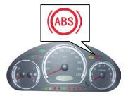
If ABS light is lit up during driving, there is a fault in ABS system With ABS not working, if the brake system functions properly, go to the nearest CHERY AUTO authorized service station for inspection.
