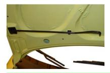
4. Press the knighthead into the clamp to avoid vibration before closing the coping.5. Lay down the coping and let it fall from about 30cm (1 inch) height. Close the coping and shake the edge of it to ensure it has been locked.
