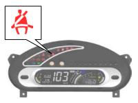
Airbag alarm indicator lamp (for the models equipped with the air bag)
