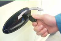
You can lock or open the door with the lock button on the side of the windows. Except the left-front door, you can lock all of the doors from outside by pressing the lock button and closing the door. When you leave the car, you can only lock the left front door from outside with the key.
