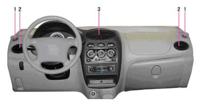
1, Front windshield defroster ventilation opening2, Side ventilation opening3, Center ventilation opening
