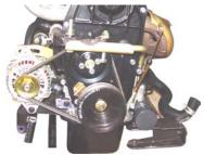
Install belt properly and ensure appropriate belt tension, otherwise generator, A/C and other system operating may be affected. If drive belt is worn, cracked or swelled, replace it.
