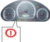
The light ON after the ignition switch turns on, and then off after about 4 s. If the light fails to light after the ignition switch turns on, or if the light doesn't extinguish after it lights, please contact the nearest special CHERY service station. If the light ON during the vehicle is traveling, it shows that the ABS has fault. If there is no ABS function while the vehicle's brake system still works as before, please get to the nearest special CHERY service station ASAP to have it examined.
