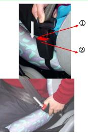
If you want to offload the seat belt, just press the red button on the ouch, the belt
