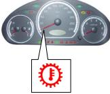
The light ON after the ignition switch turns on, and then extinguishes after about 4 s.
