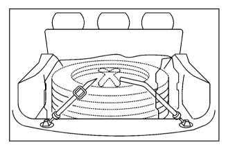
Put back all tools as they were stored in the rear storage compartment and put the compartment cover back on.
