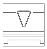
3. Find the jacking location using the hoisting notches located in the plastic molding. The notches in the plastic molding are marked with a triangle shape to help you find them.
