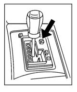
Use a tool to remove the cap with the lock symbol located next to the shift lever.
