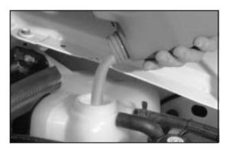
Fill the coolant surge tank with the proper mixture, to slightly above the FULL COLD/FROID line on the side of the coolant surge tank.
