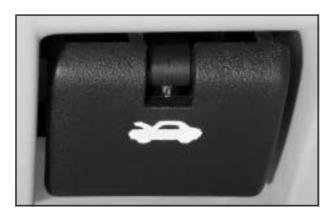
Pull the hood release lever inside the vehicle.
