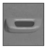
The URPA display is located inside the vehicle, above the liftgate glass. It has three color-coded lights that can be seen through the rearview mirror or by turning around.
