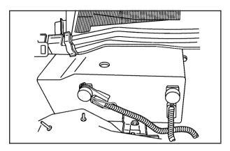
4. Open the hoods and locate the positive (+) and negative (-) terminal locations of the other vehicle, as well as the positive (+) terminal location on your vehicle's battery. See Engine Compartment Overview on page 5-12 for more information on the location of the battery.
