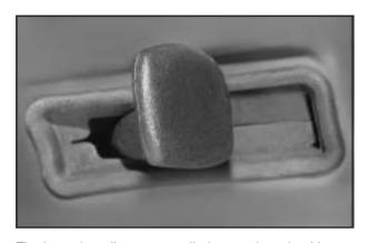
The lever that allows you to tilt the steering wheel is located on the left side of the steering column.
