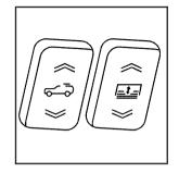
The sunroof/sunshade switches are located in the headliner between the driver and front passenger.
