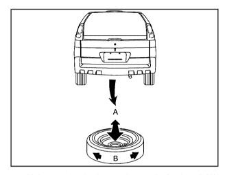
Make sure the tire is stored securely. Push, pull (A), and then try to turn the tire (B). If the tire moves, use the wheel wrench to tighten the cable.
