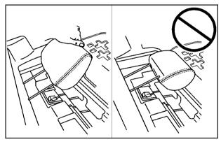
Store the head rests in the storage compartment behind the third row. Open the cover and insert the head rest posts through the slats in the storage area. The head rests must be stored with the front of the rest facing up. Position and snap the head rests in the provided storage tray.
