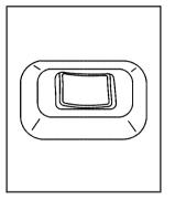
Your vehicle may have this feature. The driver's and passenger's seatback lumbar support can be adjusted by moving the control located on the outboard side of the seat cushions.
