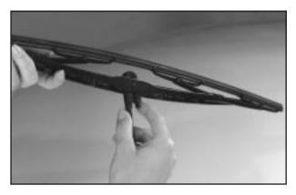
Lift the wiper blade assembly up so it is in a T-shaped position. You should be able to see a tab.
