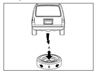
Make sure the tire is stored securely. Push, pull (A), and then try to turn (B) the tire. If the tire moves, use the lug wrench to tighten the cable.
