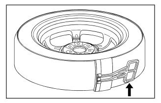
Remove the plastic spare tire heat shield by pulling the rubber latch. Store the plastic spare tire heat shield. See Storing a Flat or Spare Tire and Tools on page 5-85 for more information.
