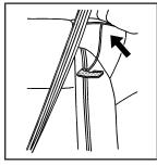
Pull the comfort guide out of its storage location and then return the headrest to its upright position.
