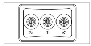
The A/V jacks, located on the rear of the floor console, allow audio or video signals to be connected from an auxiliary device such as a camcorder or a video game unit to the RSE system. Adapter connectors or cables might be required to connect the auxiliary device to the A/V jacks. Refer to the manufacturer's instructions for proper usage.
