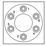
13. Tighten the wheel nuts firmly in a crisscross sequence, as shown.
