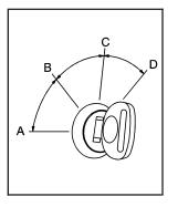
With the key in the ignition, you can turn it to four different positions.
