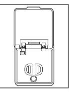
The power outlet is located on the rear of the center console.
