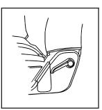
In vehicles with seats that have manual reclining seatbacks, the lever used to operate them is located on the outboard side of the seat. To recline the seatback, do the following:
