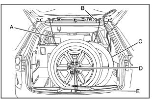
4. Pull the cable (A) through the door striker (E), the center of the wheel (D), and the plastic spare tire heat shield (C), as shown.
