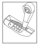
2. Press the plus/minus button located on the shift lever, to increase or decrease the gear range available based upon your current driving conditions and needs.
