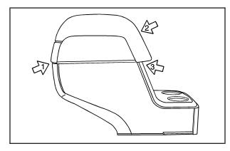
To access the upper storage area, press the upper button (2) and lift up. To access the lower storage area, press the lower button (3) and lift up. The top of the console can be folded forward for increased storage area. Lift up on handle on the rear of the console (1) and pull forward.
