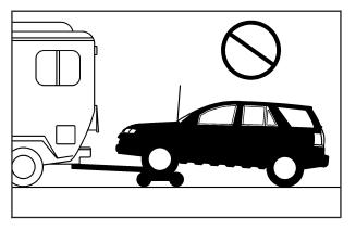
All-wheel-drive vehicles must not be towed with two wheels on the ground. To properly tow these vehicles, they should be placed on a platform trailer with all four wheels off of the ground or dinghy towed from the front. Dolly Towing (Front-Wheel-Drive Vehicles Only)
