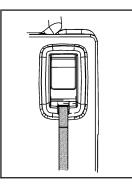
Pull up on the release lever located on the back of the seat. The headrest moves forward automatically.
