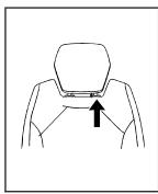
Pull the head restraint up to raise it. To lower the head restraint, press the release button, located on the head restraint post on the top of the seatback, while you push the head restraint down.
