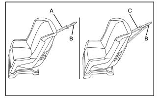
A top tether (A, C) anchors the top of the child restraint to the vehicle. A top tether anchor is built into the vehicle. The top tether attachment (B) on the child restraint connects to the top tether anchor in the vehicle in order to reduce the forward movement and rotation of the child restraint during driving or in a crash.
