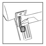
To set the parking brake, push down the parking brake pedal down with your left foot.
