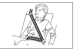
4. Buckle, position, and release the safety belt as described previously in this section. Make sure that the shoulder belt crosses the shoulder.
