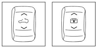
**Vent:** From the closed position, press and hold the front of the driver's side switch to vent the sunroof. Press and hold the rear of the driver's side switch to close the sunroof.
