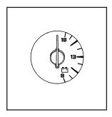
When the engine is not running, but the ignition is on, this gage shows the battery's state of charge in DC volts.
