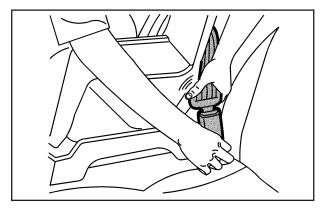
Push the latch plate into the buckle until it clicks. Make sure the release button is positioned so you would be able to unbuckle the safety belt quickly
