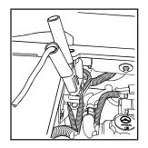
Connect the red positive (+) cable to the positive (+) terminal of the dead battery.
