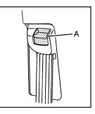
To move it down, push down on the button (A) and move the height adjuster to the desired position. You can move the height adjuster up by pushing up on the shoulder belt guide.
