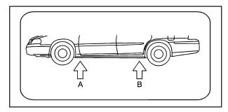
To identify the appropriate jacking location, find the triangle (A) about 12 inches (30.5 cm) from the front tire or (B) about 10.5 inches (27 cm) from the rear tire.
