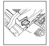
Connect the other end of the negative (-) cable at least 18 inches (45 cm) away from the dead battery, but not near engine parts that move.
