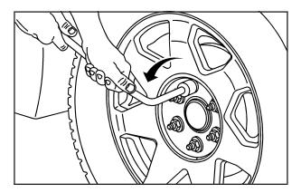
Loosen the wheel nuts — but do not remove them — using the lug wrench. For wheels with a wheel lock key, use the wheel lock key between the lock nut and lug wrench. The key is supplied in the front passenger door pocket.
