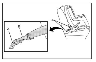
Lower anchors (A) are metal bars built into the vehicle. There are two lower anchors for each LATCH seating position that will accommodate a child restraint with lower attachments (B). **Top Tether Anchor**
