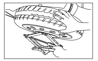
8. Disconnect the lug wrench from the jack and carefully remove the jack. Use one hand to push against the spare tire while firmly pulling the jack out from under the spare tire with the other hand.
