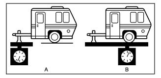
If you are using a weight-carrying hitch or a weight-distributing hitch, the trailer tongue (A) should weigh 10-15 percent of the total loaded trailer weight (B).
