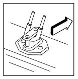
8. Make sure the metal tube is centered at the striker. Push the tube towards the front of the vehicle.
