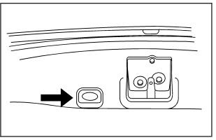
Power Liftgate Button Near Liftgate Latch
