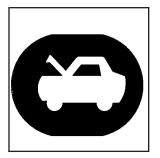
Pull the interior hood release handle with this symbol on it. It is located to the left of the steering column below the instrument panel.
