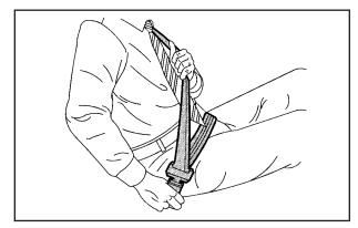
To make the lap part tight, pull down on the buckle end of the belt as you pull up on the shoulder belt.
