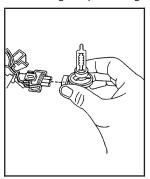
Disconnect the wire connector from the bulb by lifting the lock tab and pulling it away from the plastic base.
