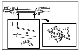
Find the jacking location using the diagram above and corresponding hoisting notches located on the underside of the vehicle's plastic molding. The notches in the plastic molding are marked with a triangle shape to help you find them.
