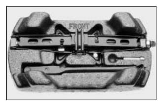
6. Turn the nut holding the jack counterclockwise and remove it. Then remove the jack and wrench.
