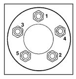
11. Tighten the wheel nuts firmly in a crisscross sequence as shown.
