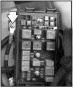
To uncover the remote positive (+) terminal, press the tab at the bottom of the fuse block and lift the cover up.
