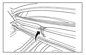
Lift the handle on the spare tire cover. The handle may hook on the front edge of the trunk's weatherstrip to hold the cover out of the way.
