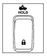
To lock or unlock all doors from inside the vehicle, use the power door lock switch located on either front door armrest.
