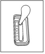
Your vehicle's automatic transaxle may have a shift lever on the steering column or on the console between the seats.
