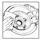
Remove any rust or dirt from the wheel bolts, mounting surfaces and spare wheel. 8. Install the compact spare tire.
