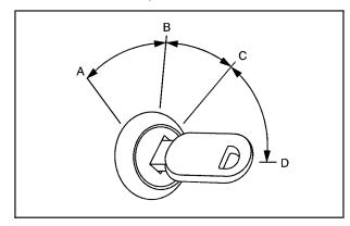
A (OFF): This is the only position in which the ignition key can be inserted or removed. This position locks the ignition and transaxle. It is a theft-deterrent feature.
