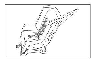
In Canada, the law requires that forward-facing child restraints have a top strap, and that the strap be anchored. In the United States, some child restraints also have a top strap. If your child restraint has a top strap, it should be anchored.
