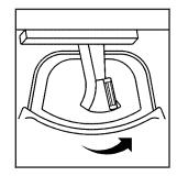
If your vehicle has the five-passenger console, there is a cupholder in front of the center console. The cupholder has an arm that adjusts to two positions to fit either a large cup or two smaller cups.
