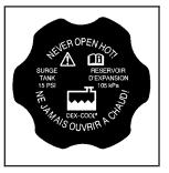
You can remove the radiator pressure cap when the cooling system, including the radiator pressure cap and upper radiator hose, is no longer hot. Turn the pressure cap slowly counterclockwise until it first stops.
