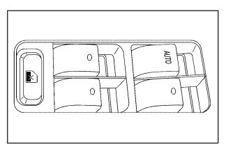
The switches on the driver's door armrest are used to control each of the windows. The power window switches work while the ignition is on, in ACCESSORY, or while Retained Accessory Power (RAP) is active. See *Retained Accessory Power (RAP)* on page 2-22. Each passenger door has its own window switch.
