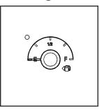
The fuel gage indicates about how much fuel is left in the fuel tank when the ignition is on.
