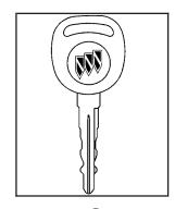
Your vehicle is equipped with PASS-Key® III (Personalized Automotive Security System) theft-deterrent system. PASS-Key® III is a passive theft-deterrent system. This means nothing special needs to be done to arm or disarm the system. It works when the key is inserted or removed from the ignition.
