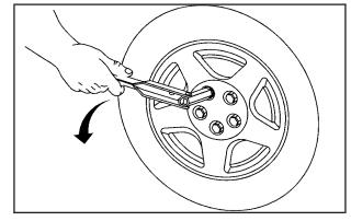
Place the wheel wrench securely over the wheel nut. Turn the wheel wrench counterclockwise to loosen all the wheel nuts, but do no remove them yet. Turn the jack handle clockwise to raise the jack lift head.
