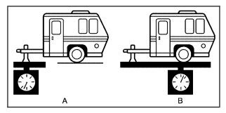
When using a weight-carrying hitch, the trailer tongue (A) should weigh 10 percent to 15 percent of the total loaded trailer weight (B).
