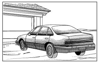
4. Turn on the low-beam headlamps and place a piece of cardboard or equivalent in front of the headlamp not being aimed. This should allow only the beam of light from the headlamp being aimed to be seen on the flat surface. Notice: Do not cover a headlamp to improve beam cut-off when aiming. Covering a headlamp may cause excessive heat build-up which may cause damage to the headlamp.
