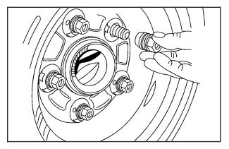
Put the wheel nuts back on with the rounded end of the nuts toward the wheel. Tighten each nut by hand until the wheel is held against the hub.
