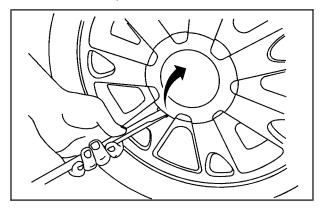
To remove a center cap, use the wrench to pry gently at the notch on the cap. Do not use a tool that is narrower than the wrench to pry at this notch. Then pry off the cap. Use the wheel wrench to loosen the plastic nut caps in a counterclockwise direction. If needed, finish loosening them by hand. The nut caps will not come off.
