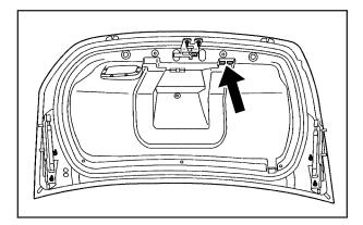
Your vehicle has a tie-down feature inside the trunk lid that can be used to secure the trunk lid when large items are stored in the trunk.
