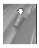
Pull forward on the seatback tab located on the outboard side of the rear seat cushion to fold the seatback down.
