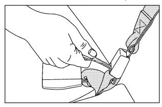
Disconnect the rear center lap-shoulder belt latch, if equipped, by using a pointed object to press the release button.
