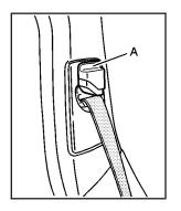
To move it down, push down on the release lever (A) move the height adjuster to the desired position. You can move the adjuster up just by pushing up on the shoulder belt guide.
