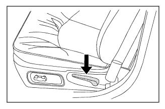
Lift the lever located on the outboard side of the seat to release the seatback, then move the seatback to the desired position. Release the lever to lock the seatback in place.
