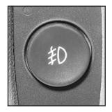
The fog lamp button is located on the instrument panel to the right of the exterior lamps knob.
