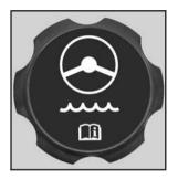
The power steering fluid reservoir is located in the engine compartment. It is on the passenger's side of vehicles with the L6 engine and is on the driver's side of vehicles with the V8 engine. See *Engine Compartment Overview on page 5-14* for reservoir location.
