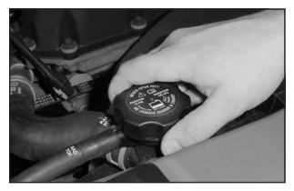
You can remove the radiator pressure cap when the cooling system, including the radiator pressure cap and upper radiator hose, is no longer hot. Turn the pressure cap slowly counterclockwise about one full turn.
