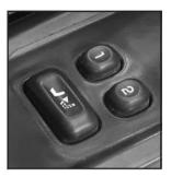
The memory seat controls are located on the driver's door, and are used to program and recall memory settings for the driver's seating positions, outside mirror positions and adjustable pedals (if equipped).
