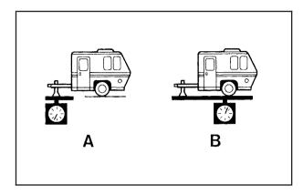
The trailer tongue weight (A) should be 10 percent to 15 percent of the total loaded trailer weight, up to a maximum or 400 lbs. (181 kg) with a weight carrying hitch. The trailer tongue weight (A) should be 10 percent to 15 percent of the total loaded trailer weight, up to a maximum of 900 lbs. (408 kg) with a weight distributing hitch.
