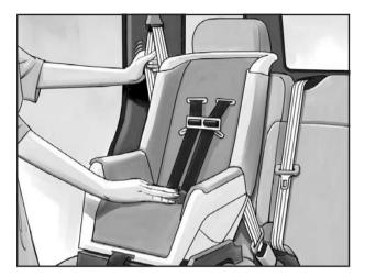
5. To tighten the belt, push down on the child restraint, pull the shoulder portion of the belt to tighten the lap portion of the belt and feed the shoulder belt back into the retractor. If you are using a forward-facing child restraint, you may find it helpful to use your knee to push down on the child restraint as you tighten the belt. 6. Push and pull the child restraint in different directions to be sure it is secure.
