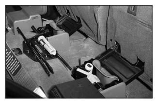
The jacking equipment you will need is stored under the rear seat on the passenger's side of the vehicle. See *Rear Seat Operation on page 1-5.* To release the jack from its holder, turn the knob on the jack counterclockwise to lower the jack head.
