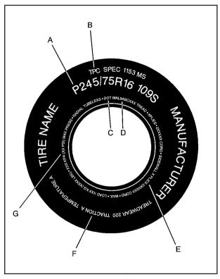
(A) Tire Size Code: The tire size code is a combination of letters and numbers used to define a particular tire's width, height, aspect ratio, construction type and service description. See the "Tire Size Code" illustration later in this section for more detail.
