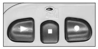
• (Record): To record a message, press this button and begin speaking. Press the button again to stop recording. You may also press and hold this button while you are speaking and then let it go when you are finished. ▷ (Play): To play a recorded message, press this button. Pressing the button more than once will return you to previously recorded messages. If you press and hold this button for more than one second, all of the recorded messages will be played back.
