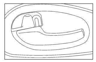
You can lock or unlock the door from the inside by sliding the manual lever forward or rearward.
