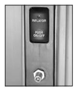
The air inflator is located in the rear compartment on the passenger's side of the vehicle behind an access cover. To remove the cover, pull the two tabs on the cover and pull it off.
