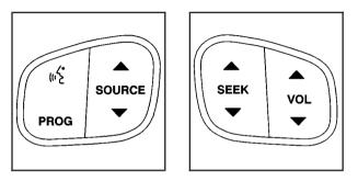
(**Constar/Voice Recognition):** If your vehicle has OnStar<sup>®</sup>, you can press this button to interact with the OnStar<sup>®</sup> system. See the OnStar<sup>®</sup> manual provided with your vehicle for more information.
