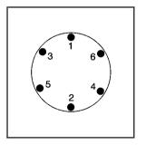
12. Use the wheel wrench to tighten the wheel nuts firmly in a crisscross sequence as shown.
