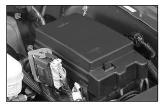
The fuse block is located under the hood in the engine compartment on the driver's side of the vehicle. See *Engine Compartment Overview on page 5-14* for more information on location.
