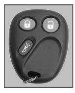
**Q** (Unlock): When you press unlock, the driver's door will unlock automatically, the parking lamps may flash and the interior lights will go on.
