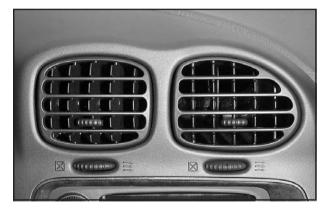
Your vehicle has air outlets that allow you to adjust the direction and amount of airflow inside the vehicle. Move the control in the center of each outlet side-to-side to direct the air from the outlet. Use the thumbwheel under the outlet to close the louvers. For the most efficient airflow and temperature control, keep the louvers in the fully opened position.
