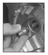
Put the nuts on by hand. Make sure the rounded end is toward the wheel.
