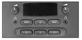
The left button with the fan symbol regulates the fan speed. The right button is used to change the direction of airflow (upper, bi-level or floor) to the rear seat area. To turn the rear climate controls on or off, press the middle button. The rear control will only turn on if the front is on and is not in defrost mode.
