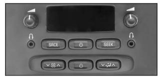
(Power): Press this button to turn the rear seat audio system on or off. The rear speakers will be muted when the power is turned on unless you have a Bose<sup>®</sup> equipped vehicle. You may operate the rear seat audio functions even when the primary radio power is off.
