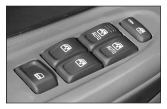
The controls for the power windows are located on the armrest on each of the side doors. With power windows, the switches operate the windows when the ignition is in RUN, ACCESSORY or when Retained Accessory Power (RAP) is active. The driver's door has a switch for each of the passenger's windows as well.
