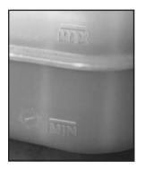
Just look at the brake fluid reservoir. The fluid level should be above MIN. If it is not, have your brake system checked to see if there is a leak.
