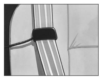
3. Be sure that the belt is not twisted and it lies flat. The elastic cord must be under the belt and the guide on top.
