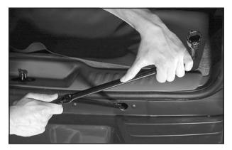
To remove the underbody-mounted spare, insert the socket end of the extension on a 45° angle downward into the hoist drive shaft hole. This will be exposed when the rear gate is open and is just above the rear bumper. Be sure the socket end of the extension connects to the hoist shaft. 2. Turn the wheel wrench counterclockwise to lower the spare tire. Keep turning the wheel wrench until the spare tire can be pulled out from under the vehicle.
