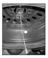
1. Check under the vehicle to see if the cable is visible.
