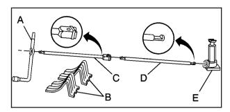
The tools you'll be using include the wheel wrench (A), wheel blocks (B), extension (socket end) (C), handle (jack end) (D), and jack (E).
