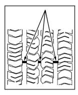
One way to tell when it's time for new tires is to check the treadwear indicators, which will appear when your tires have only 1/16 inch (1.6 mm) or less of tread remaining. Some commercial truck tires may not have treadwear indicators. You need a new tire if any of the following statements are true:
