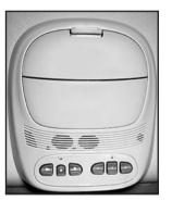
The overhead console includes sunglasses storage, a HomeLink<sup>®</sup> transmitter and a Travel Note recorder.
