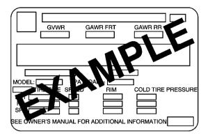
The Certification/Tire label is found on the driver's door edge, above the door latch. The label shows the size of your original tires and the inflation pressures needed to obtain the gross weight capacity of your vehicle. This is called the Gross Vehicle Weight Rating (GVWR). The GVWR includes the weight of the vehicle, all occupants, fuel, cargo and trailer tongue weight, if pulling a trailer.
