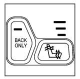
Your vehicle may have heated front seats. The buttons used to control this feature are located on the front door armrests. The engine must be running for the heated seat feature to work. To heat only the seatback, press the button with the words BACK ONLY. An indicator light on the switch will glow to designate that only the seatback is being heated. Additional presses will cycle through the heat levels for the seatback only. Press the horizontal button again to heat the whole seat.
