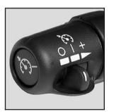
The cruise controls are located on the end of the turn signal/multifunction lever.
