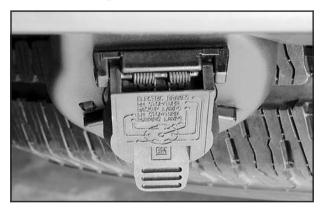
Your vehicle is equipped with a seven-wire trailer towing harness. This harness has a seven-pin universal heavy-duty trailer connector that is attached to a bracket on the hitch platform. The seven-wire harness contains the following trailer circuits:
