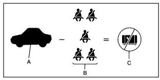
Refer to your vehicle's tire and loading information label for specific information about your vehicle's capacity weight and seating positions. The combined weight of the driver, passengers and cargo should never exceed your vehicle's capacity weight.
