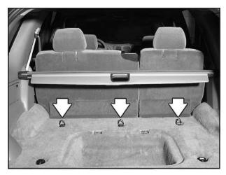
Anchor brackets for the rear seat positions are located on the floor in the cargo area of your vehicle. Do not use the rear tie-down brackets near the liftgate for top strap tethers. Do not use a child restraint with a top strap in the right front passenger's position because there is no place to anchor the top strap.
