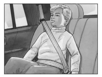
4. Buckle, position and release the safety belt as described in *Rear Seat Passengers on page 1-20.* Make sure that the shoulder belt crosses the shoulder.
