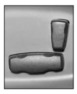
The power seat controls are located on the outboard side of the front seat cushions. The horizontal control adjusts the seat cushion and the vertical control adjusts the seatback.
