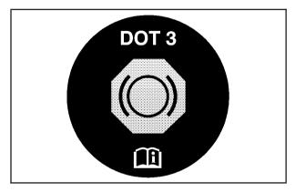
Your brake master cylinder reservoir is filled with DOT-3 brake fluid. See *Engine Compartment Overview on page 5-14* for the location of the reservoir.
