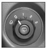
This control is located to the right of the steering wheel on the instrument panel. To turn the rear wiper on, turn the control to either 1, 2, or 3. For delayed wiping, turn the control to 1 or 2. For steady wiping, turn the control to 3. To turn the wiper off, turn the control to 0.
