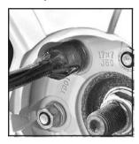
Using the wheel wrench, loosen all the wheel nuts. Don't remove them yet.
