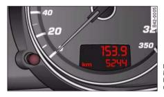
Fig. 5 Detail of the instrument cluster: Mileage recorder with reset button
