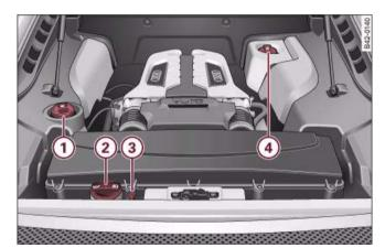
Fig. 116 Typical locations of fluid containers, engine oil dipstick and engine oil filler cap
