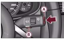
Fig. 8 Windscreen wiper lever: Reset button and rocker switch
