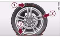
Fig. 124 The Tyre Mobility System is NOT suitable for repairing this type of damage to tyres.
