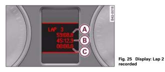
Each time you press the top part of the rocker switch when the lap timer is running, the current lap time is stored and the next lap time is started simultaneously. Simply repeat this procedure to record subsequent laps.
