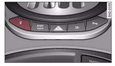
Fig. 76 Centre console: Switch for Audi magnetic ride
