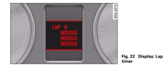
With the ignition switched on, keep pressing the RESET button (B) ⇒ fig. 21 until the lap timer ⇒ fig. 22 appears.
