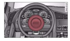
Fig. 95 Driver's airbag in steering wheel
