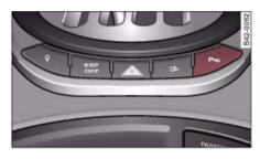
Fig. 74 Parking aid switch in centre console
