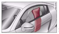
Fig. 100 Side airbag in inflated condition
