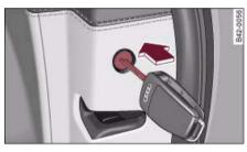
Fig. 39 Locking the door manually
