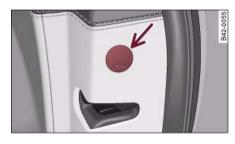
Fig. 38 Manual locking device on the passenger's door pillar
