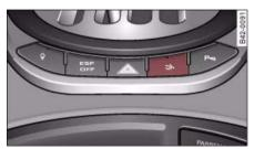
Fig. 111 Switch for rear spoiler
