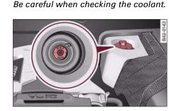
Fig. 120 Engine compartment: Markings on radiator expansion tank
