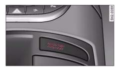
Fig. 102 Lamp indicates that front passenger's airbag has been deactivated via key-operated switch
