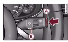
Fig. 12 Windscreen wiper lever: Controls for menu display
