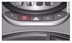
Fig. 110 Centre console with ESP switch
