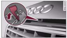
Fig. 41 Luggage lid unlocked: Release lever
