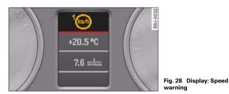
The speed warning function will warn you if the vehicle exceeds the pre-set maximum speed. The system gives an audible warning signal if the set speed is exceeded by about 10 km/h. A warning symbol will also appear in the display  $\Rightarrow$  fig. 28.
