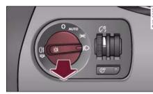
Fig. 46 Detail of the dashboard: Light switch
