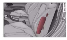
Fig. 99 Location of side airbag in driver's seat
