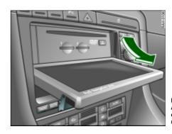
Fig. 5 Display open: Access to the DVD drive and the MP3 card reader
