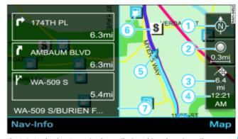
Fig. 151 Navigation: Example of map display with activated turn list
