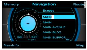
Fig. 126 Navigation: Entering a street as destination using the speller
