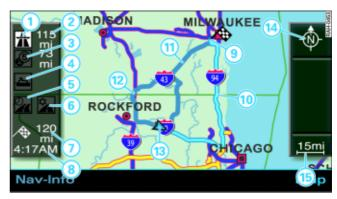
Fig. 136 Navigation: Example of map display after route has been calculated
