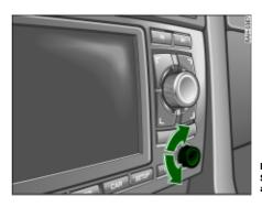
Fig. 14 Navigation System ON/OFF knob adjusting volume
