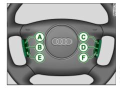
Fig. 17 Multi-function steering wheel with audio operation (version A)
