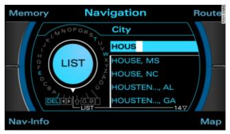
Fig. 124 Navigation: Entering the destination using the speller
