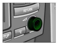
Fig. 15 Navigation System ON/OFF knob
