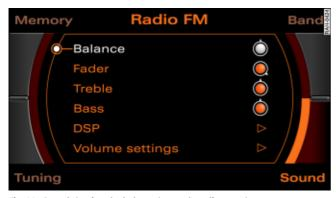
Fig. 96 Sound: Setting the balance (example radio menu)
