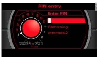
Fig. 6 Speller display: Entering PIN
