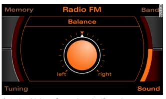
Fig. 97 Sound: Balance adjustment (example radio menu)
