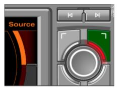
Fig. 11 Navigation System: Assignment of control buttons and button symbols to the screen corners.
