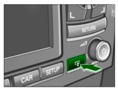
Fig. 4 Navigation System: Button for opening and closing the display
