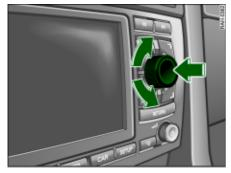
Fig. 9 Navigation System: Control knob
