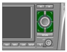
Fig. 10 Navigation System: Control buttons
