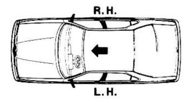
However, working on engine on bench, right and left side are referred to an operator looking at the engine from the flywheel side, as illustrated below:
