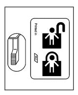
Move the lever down to engage the security lock. Move the lever up to disengage the security lock. The rear doors of your vehicle cannot be opened from the inside while this feature is in use. If you want to open the rear door while the security lock is on, unlock the door and open the door from the outside.
