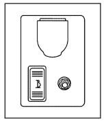
The accessory inflator is located in the rear compartment on the driver's side of the vehicle, behind an access cover, and near the liftgate opening.
