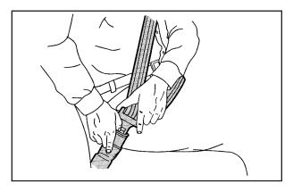
To unlatch the belt, push the button on the buckle.
