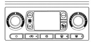
With this system you can control the heating, cooling and ventilation for your vehicle. When your vehicle is first started and the climate control system is on, or if the climate control system has been turned on, the display will show the driver's temperature setting for five seconds. Then it will show the outside temperature.
