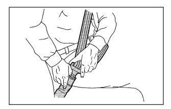
To unlatch the belt, push the button on the buckle. The belt should go back out of the way.
