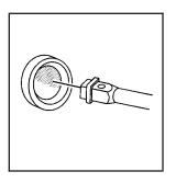
11. If the spare tire is hanging from the cable, insert the socket end of the extension into the hoist shaft hole on a 45 degree angle downward. 12. Be sure that the socket end of the extension connects to the hoist shaft.
