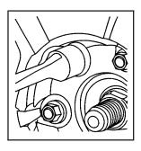
Using the wheel wrench, loosen all the wheel nuts.
