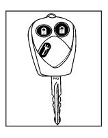
This vehicle has double-sided keys that can be used for the ignition and door lock.
