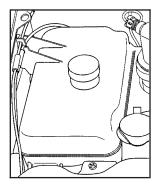
The coolant level should be at least up to the FULL COLD mark. If it is not, you may have a leak at the pressure cap or in the radiator hoses, heater hoses, radiator, water pump, or somewhere else in the cooling system.
