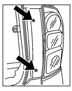
2. Remove the screws from the taillamp assembly.
