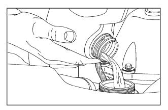
Fill the radiator with the proper DEX-COOL®
