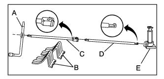
The tools you will be using include the wheel wrench (A), wheel blocks (B), extension(s), (socket end) (C), handle (jack end) (D), and jack (E).
