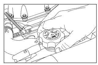
1. You can remove the radiator pressure cap when the cooling system, including the radiator pressure cap and upper radiator hose, is no longer hot.
