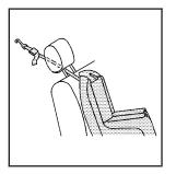
Fold down the head restraint and route the single tether under the head restraint and in between the head restraint posts. See Rear Seat Operation on page 16.
