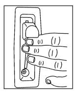
Lift the lever, located on the outboard side of the seatback, and fold the seatback forward.
