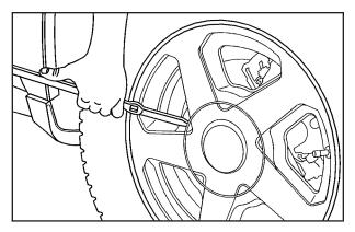
1. If your vehicle has a wheel cap that covers the wheel nuts, position the chisel end of the wheel wrench in the notch and pry it off.
