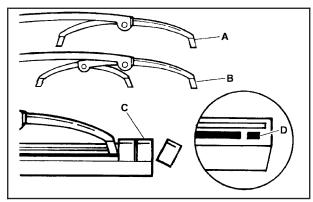
4. To install the new wiper insert, slide the insert (D), notched end last, into the end with two blade claws (A). Slide the insert all the way through the blade claws at the opposite end (B). The plastic caps (C) will be forced off as the insert is fully inserted.
