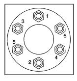
13. Use the wrench to tighten the wheel nuts firmly in a crisscross sequence as shown.
