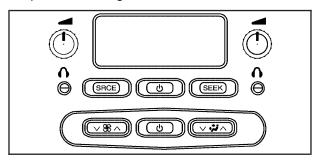
$V \mathcal{R} \wedge (Fan)$  Press this button to adjust the fan speed.
