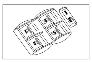
The controls for the power windows are located on the armrest on each of the side doors. With power windows, the switches operate the windows when the ignition is in RUN, ACC or when Retained Accessory Power (RAP) is active. See *Retained Accessory Power (RAP)* on page 108. The driver's door also has a switch for each of the passenger's windows.
