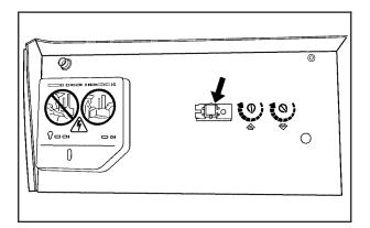
Go to the garage. Locate the garage door motor head and press and release the "learn" button.
