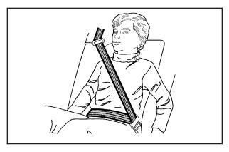
4. Buckle, position, and release the safety belt as described in *Rear Seat Passengers on page 32*. Make sure that the shoulder belt crosses the shoulder.
