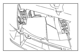
Pull the headlamp assembly away from the vehicle to access the electrical connectors. 4. Remove the bulb cover for the high beam (A) and low beam (B) bulbs.
