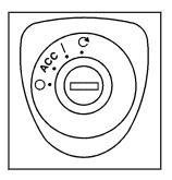
Use the key to turn the ignition switch to four different positions. The ignition switch is located on the center console.
