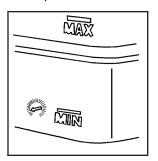
Look at the brake fluid reservoir. The fluid level should be above MIN. If it is not, have your brake system checked to see if there is a leak.
