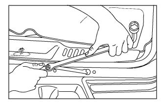
Turn the wheel wrench counterclockwise to lower the spare tire. Keep turning the wheel wrench until the spare tire can be pulled out from under the vehicle.
