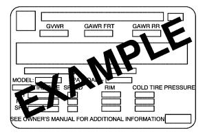
A vehicle specific Certification/Tire label is found on the rear edge of the driver's door. The label shows the size of your vehicle's original tires and the inflation pressures needed to obtain the gross weight capacity of your vehicle.
