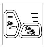
Your vehicle has heated front seats. The buttons used to control this feature are located on the front door armrests. The engine must be running for the heated seat feature to work.
