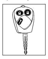
a (Unlock): Press the unlock button to automatically unlock the driver's door. The parking lamps may flash and the interior lights will go on. Press the unlock button again and all remaining doors will unlock.
