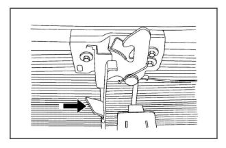
2. Then go to the front of the vehicle and push the secondary hood latch up and to the right to release it, then lift the hood.
