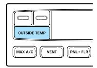
If the selected temperature is changed while the outside temperature is displayed, the new temperature will be displayed for four seconds after it is changed, then the outside temperature will return to the window.
