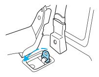
3. Use the black plastic clip (located just above the detachable anchor) to stow the loose seat belt.
