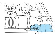
If the engine coolant has not been checked for a long period of time, the engine coolant reservoir may eventually empty. If this occurs, add engine
