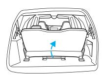
When reinstalling a rear seat in your vehicle it must be placed in its original position. Improper installation of the seat will prevent correct use of the safety belts and could increase the risk of injury. Refer to the warning label on the seat belt.
