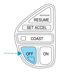
Once speed control is switched off, the previously programmed set speed will be erased.
