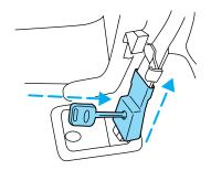
2. Before removing the seat, be sure that the detachable anchor tongue is stowed flat into the vehicle floor.
