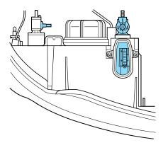
vehicle is not positioned on a level surface, the slope will be included in the vertical indication. Therefore, vertical and horizontal headlamp adjustment should be performed only when the beam direction appears to be incorrect.
