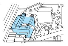
in each cell up to the "level" indicator. Do not overfill the battery cells.
