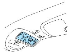
In order for the auxiliary A/C-heater controls to function, the driver's auxiliary A/C-heater control must be set to REAR.
