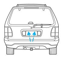
Make sure that the liftgate door and/or window are closed to prevent exhaust fumes from being drawn into the vehicle. This will also prevent passengers and cargo from falling out. If you must drive with the liftgate door or window open, keep the vents open so outside air comes into the vehicle.
