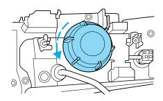
6. Disconnect the electrical connector from the headlamp bulb by grasping the wire and pulling it rearward.
