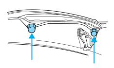
2. Carefully pull the lamp assembly outward to expose the electrical connector.
