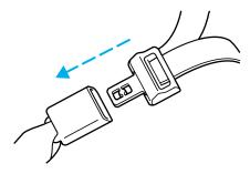
2. To unfasten, push the red release button and remove the tongue from the buckle.
