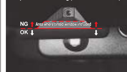
Part prohibited for tinting (FCM detection area)
