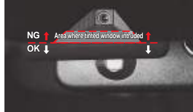
Part prohibited for tinting (FCM detection area)
