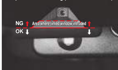
Part prohibited for tinting (FCM detection area)
